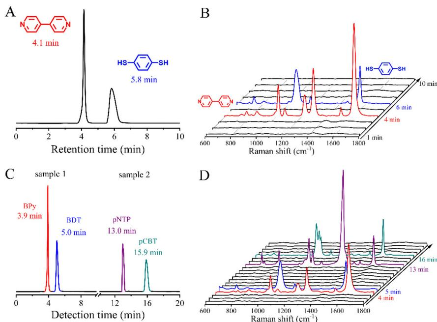
**Fig. 1** Chromatogram (A) and time-dependent SERS spectra (B) of the two-component mixture containing 4,4'-bipyridine and 1,4-benzenedithiol. Chromatogram (C) and time-dependent SERS spectra (D) of two continuously detected two-component mixtures. The interval time is one minute. The second sample is injected immediately after the detection of the first sample is finished.
