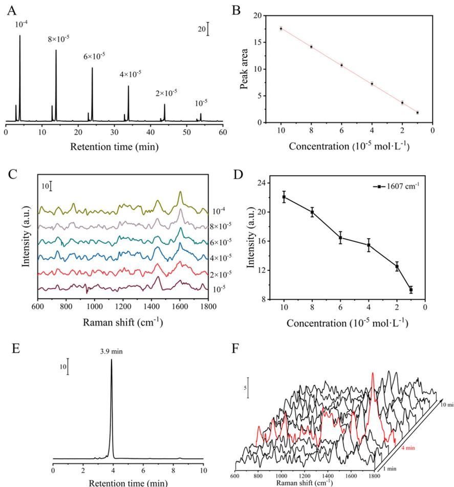
**Fig. 3** Chromatogram (A) and SERS spectra (C) of rosiglitazone maleate at different concentrations. (B) HPLC standard curve of rosiglitazone maleate. (D) Relation curve between the SERS intensity and concentration of rosiglitazone maleate. Chromatogram (E) and time-dependent SERS spectra (F) of the rosiglitazone tablet. The interval time is one minute.
