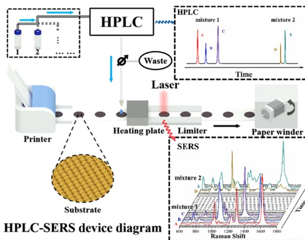
Scheme 1 Schematic diagram of the HPLC-SERS hyphenated system.
