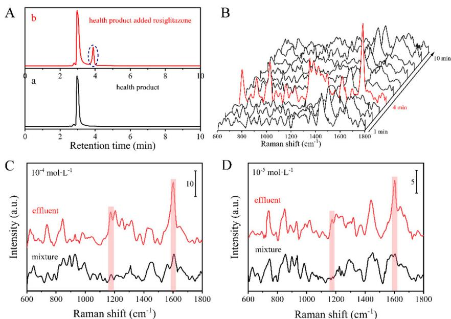
**Fig. 4** (A) Chromatograms of health products with (b) and without rosiglitazone (a). (B) Time-dependent SERS spectra of health products spiked with rosiglitazone. The interval time is one minute. Mixture and effluent of health products containing rosiglitazone at a concentration of  $10^{-4}$  mol  $\text{dm}^{-3}$  (C) and  $10^{-5}$  mol  $\text{dm}^{-3}$  (D).
