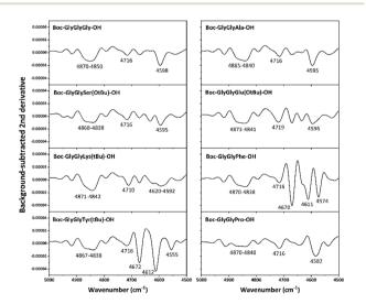
Fig. 3 The background-subtracted second derivative spectra in the 5000-4500 cm<sup>-1</sup> region for 200 mM solution of eight amino acids in DMSO.
