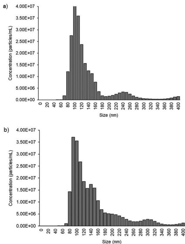
**Fig. 4** Exosome quantification by NTA. (a) Exosome distribution derived from CA125(+) OVCAR3. The total concentration of exosomes present in the 1:4 diluted sample is  $4.93 \pm 0.16 \times 10^8$  exosomes per mL. (b) Exosome distribution derived from CA125(-) Met-5a. The total concentration of exosomes presents in the 1:4 diluted sample is  $1.83 \pm 0.65 \times 10^8$  exosomes per mL.
