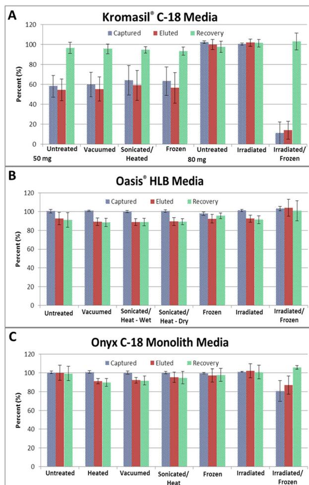
**Fig. 1** Results from testing of reverse phase media treated with specified stress conditions – (A) Kromasil® C-18; (B) Oasis® HLB; (C) Onyx C18 monolith guard column. Error bars represent actual standard deviations for each set of experiments.
