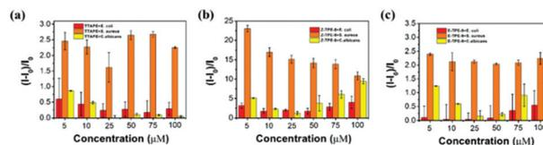
Fig. 3 Histograms of the fluorescence ratio of different concentrations of (a) TTAPE, (b) Z-TPE-9 and (c) E-TPE-9 bound with three microorganisms.  $I$  is the fluorescence intensity value of TPEs with the addition of microorganisms at 461 nm and  $I_0$  is the fluorescence intensity value of TPEs alone at 461 nm at the same concentration.)
