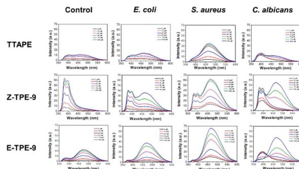
**Fig. 1** Fluorescence spectra of TTAPE, Z-TPE-9 and E-TPE-9 (5, 10, 25, 50, 75, and 100  $\mu$ M) with the addition of Amp<sup>r</sup> *E. coli*, *S. aureus* and *C. albicans* after 30 min of incubation, respectively.
