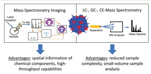
Fig. 2 Mass spectrometry (MS) techniques using organoid samples. Advantages for using mass spectrometry imaging and liquid chromatography (LC)-, gas chromatography (GC)-, and capillary electrophoresis (CE)-MS to measure the chemical components of three-dimensional organoid samples are compared.
