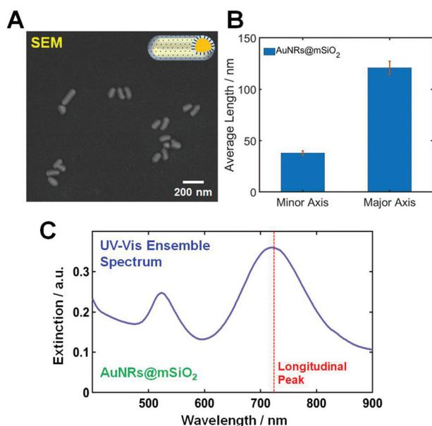
Fig. 1 (A) SEM image of AuNRs@mSiO<sub>2</sub>. (B) Histogram showing the size distribution of AuNRs@mSiO<sub>2</sub>. (C) UV-Vis extinction spectrum of AuNRs@mSiO<sub>2</sub>. The red-dotted line indicates the position of the longitudinal LSPR peak.
