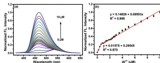
**Fig. 2** (a) Normalized fluorescence intensity spectra of the probe BTD (10  $\mu\text{M}$ ) in the presence of 0–10  $\mu\text{M}$   $\text{Al}^{3+}$  in pure water (containing 1% DMSO). (b) The linear changes in the normalized fluorescence intensity at 470 nm of the probe BTD and as a function of  $\text{Al}^{3+}$  concentration.  $\lambda_{\text{ex}} = 345$  nm, slit (nm): 2.5/2.5.
