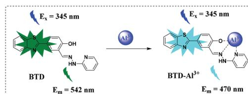
**Scheme 1** Proposed mechanism for sensing Al<sup>3+</sup>.
