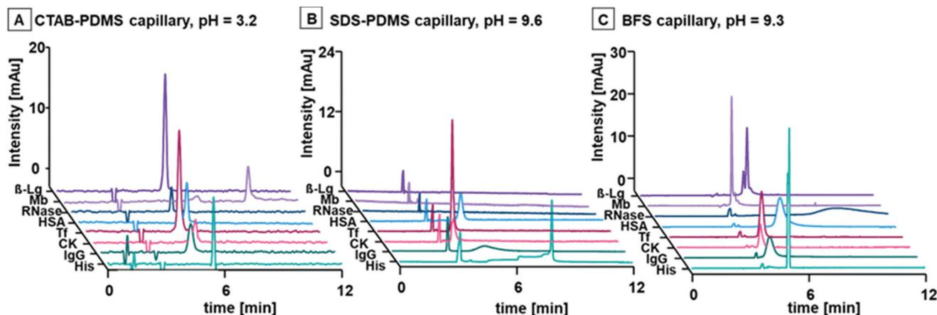
Fig. 4 CE analysis of eight model analytes with various MWs and  $pI$ s at low (A, CTAB-PDMS capillary) and high pH (B, SDS-PDMS capillary; C, BFS capillary). A fast EOF and symmetrical peaks for all analytes were produced with the CTAB-PDMS capillary (A). The peaks HSA, Tf and CK were symmetrical and adsorption free with the SDS capillary (B). The BFS capillary was superior for all other analytes with a sufficient separation efficiency for the isoforms  $\beta$ -Lg A and  $\beta$ -Lg B (C).
