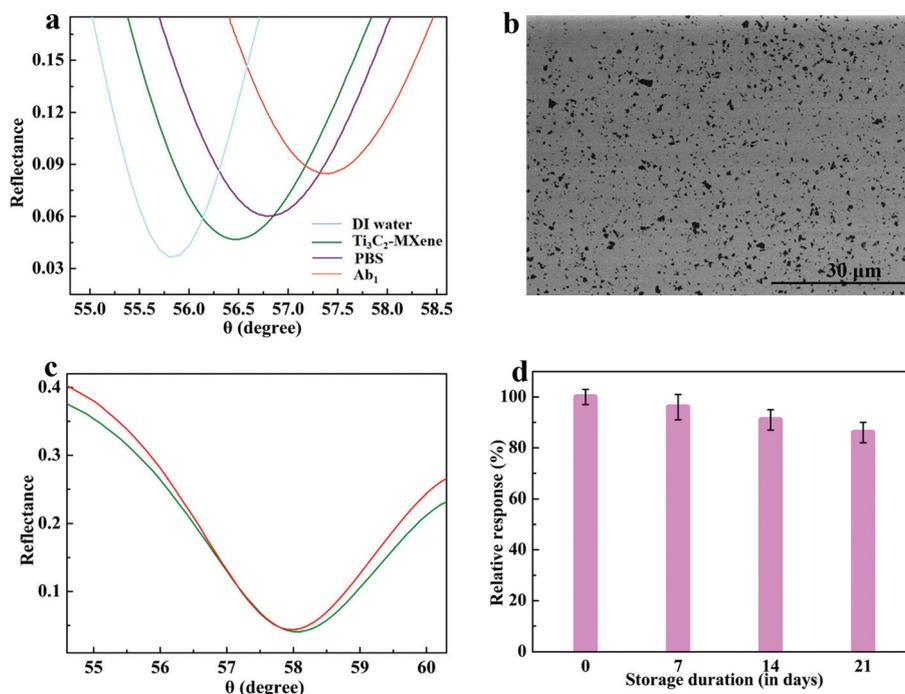
Fig. 4 The resonant angle changes before and after assembling Ti<sub>3</sub>C<sub>2</sub>-MXene nanosheets and the immobilization of Ab<sub>1</sub> (a), SEM image of Ti<sub>3</sub>C<sub>2</sub>-MXene nanosheets modified gold film (b), SPR spectra of the prepared sensing platform before and after 10 times washing with DI water (c), and stability measurement of the Ti<sub>3</sub>C<sub>2</sub>-MXene-based sensing platform (d). Error bar =  $\pm$ S.D. and  $n = 3$ .
