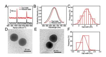
Fig. 2 Detection mechanism. (A) Raman spectra and (B) the corresponding scattering spectra of the individual core-satellite assembly in the absence and presence of 100 nM  $\rm Hg^{2+}$ . Typical TEM image of the isolated gold dimer (D) before and (E) after treatment with excess  $\rm Hg^{2+}$ . Statistical analysis of gap width in the (C) absence and (F) presence of excess  $\rm Hg^{2+}$ .
