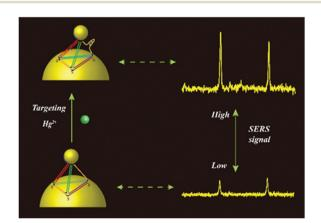
Scheme 1 Schematic of the mechanism of Hg<sup>2+</sup> detection.
