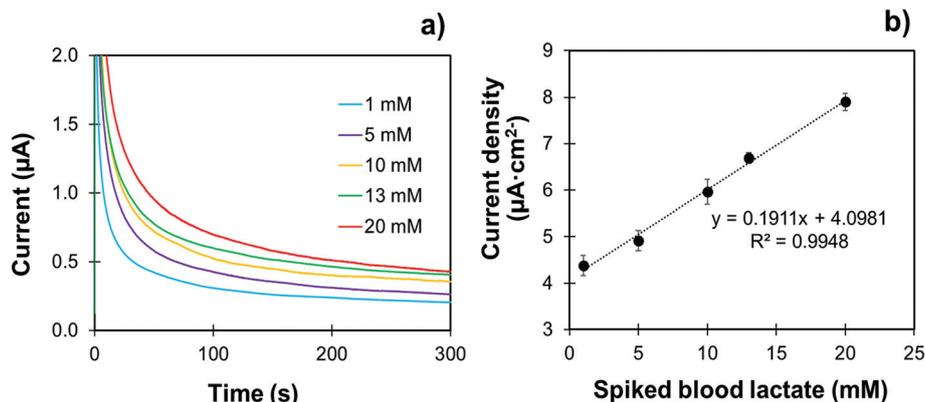
Fig. 2 Amperometric responses of the TiO<sub>2</sub> sol-G nanocomposite/SPCEs ( $n = 5$ ) for various spiked lactate concentrations (0.001–0.020 M) in whole blood measured at +0.5 V (a). Calibration plot for blood lactate detection constructed from the signal measurements presented in (a) (b).
