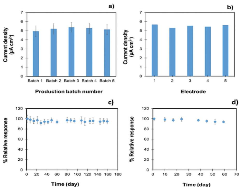
Fig. 3 Reproducibility of five different nanocomposite production batches (a) and TiO<sub>2</sub> sol-G nanocomposite modified electrodes (b). Long-term stability of the TiO<sub>2</sub> sol-G nanocomposite (c) and the nanocomposite modified electrodes (d) recorded in 0.1 M PB (pH 7.4) containing 5 mM lactate at +0.5 V; each data point for a, c, and d has been obtained by measurements with 5 individual electrodes; error bars indicate the standard deviations.
