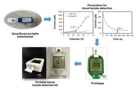
Fig. 4 Steps for developing a portable blood lactate electrochemical device.
