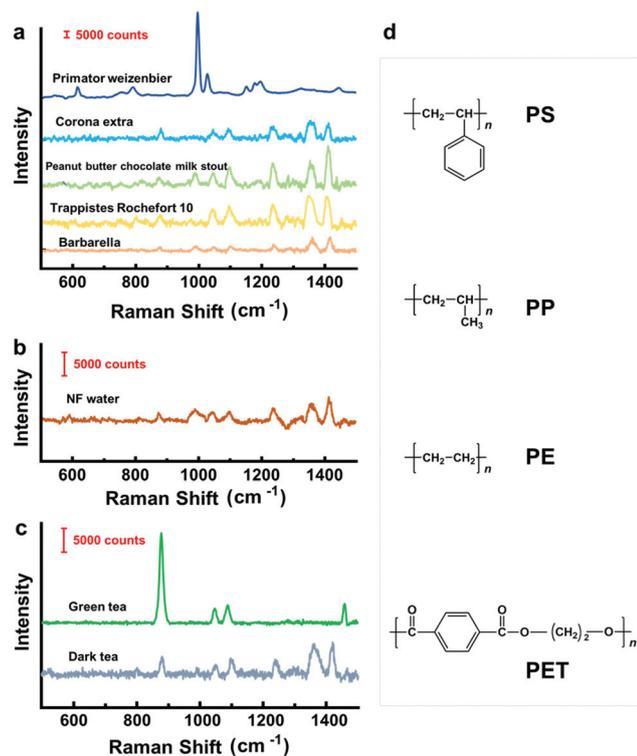
Fig. 4 Identification of chemical compositions of microplastics. (a–c) Raman spectroscopic characterizations of microplastics extracted from beers (a), mineral water (b) and teas (c). Histograms showing the number of microplastics in various beverages. (d) Chemical structures of the various plastics for reference.
