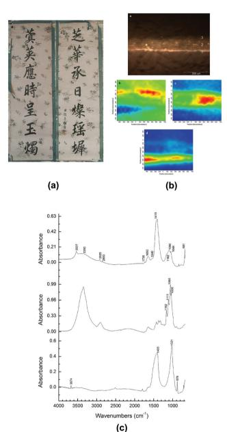
Fig. 7 (a) The piece of calligraphy Tie Luo (132.5 cm × 42 cm, which uses the Fen Jian with coloured pigment coating. (b) Micrograph (top) and ATR-FTIR mapping of cross-section of Tie Luo shows chemical distributions of pigment layer (middle left), paper fibre (middle right) and ground ash (bottom). (c) ATR-FTIR spectra of different locations in pigment layer (top), paper fibre layer (middle) and ground ash layer (bottom). Reproduced with permission, 122 copyright (2018) Springer Nature.
