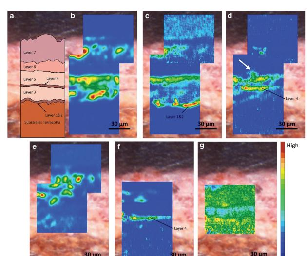
Fig. 4 (a) Optical microscopic image of the cross section from the 7-layer painted materials on the terracotta statue. Chemical images displaying the distribution of (b) lead white, (c) lipid—siccative oil, (d) lead carboxylates, (e) gypsum, (f) protein, and (g) calcium oxalates. Reprinted with permission, <sup>94</sup> copyright (2020) Springer Nature.
