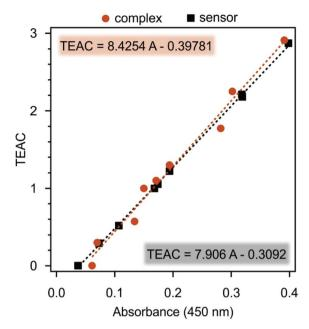
Fig. 3 TEAC values plotted against the absorbance recorded at 450 nm wavelength and 10 µM antioxidant concentration. The dashed lines are linear fits to the data.
