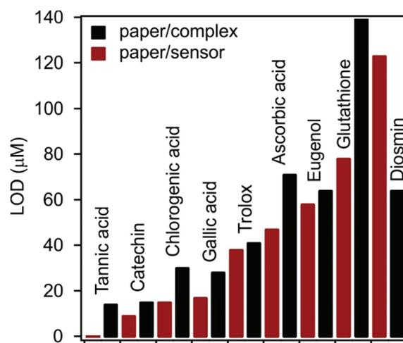
Fig. 5 LOD values determined for the antioxidants by sensor measurements. P-Cu(Nc)<sub>2</sub>: paper/complex and P-dLDH-Alg-Cu(Nc)<sub>2</sub>: paper/sensor.
