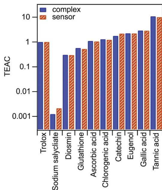
Fig. 2 TEAC values determined by Cu(Nc)<sub>2</sub> (complex) and dLDH-Alg-Cu(Nc)<sub>2</sub> (sensor) for different molecular antioxidants using eqn (4).
