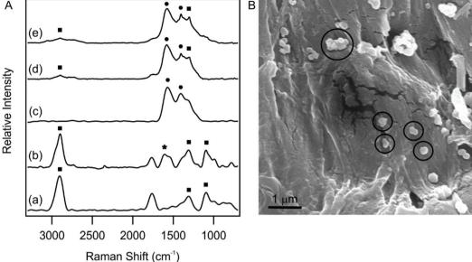
Fig. 4 (A) SERS spectra of cellulose filter paper (a), P-dLDH (b),  $Cu(Nc)_2$  (c),  $P-Cu(Nc)_2$  (d) and  $P-dLDH-Alg-Cu(Nc)_2$  (e). Squares ( $\blacksquare$ ) refer to the peaks of the paper substrate, stars ( $\star$ ) for dLDH and circles ( $\bullet$ ) for  $Cu(Nc)_2$ . (B) SEM image of  $P-dLDH-Alg-Cu(Nc)_2$ . The empty circles in (B) indicate the position of dLDH particles.
