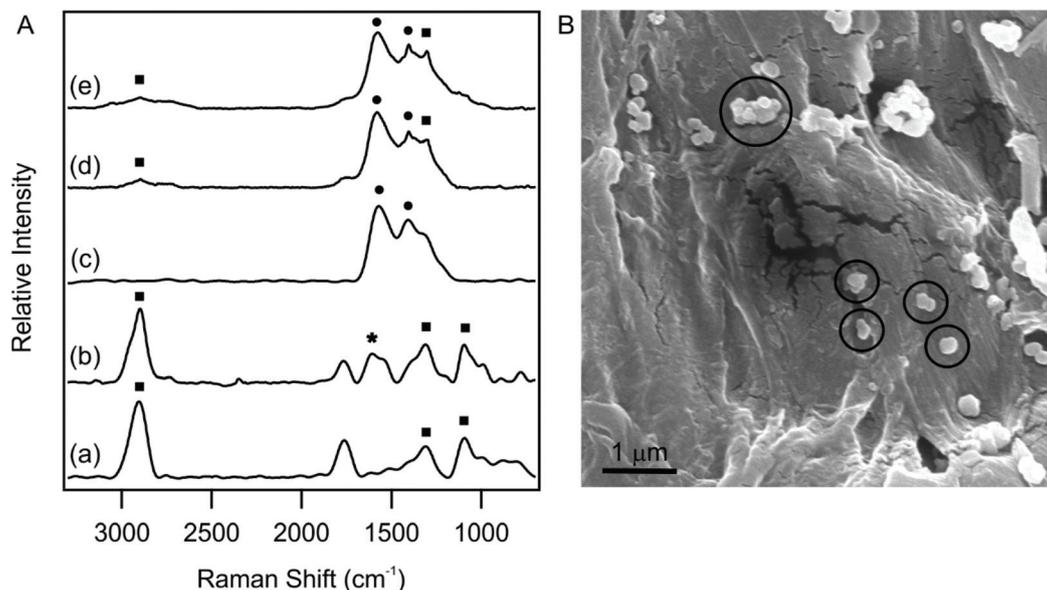
Fig. 4 (A) SERS spectra of cellulose filter paper (a), P-dLDH (b), Cu(Nc)<sub>2</sub> (c), P-Cu(Nc)<sub>2</sub> (d) and P-dLDH-Alg-Cu(Nc)<sub>2</sub> (e). Squares (■) refer to the peaks of the paper substrate, stars (★) for dLDH and circles (●) for Cu(Nc)<sub>2</sub>. (B) SEM image of P-dLDH-Alg-Cu(Nc)<sub>2</sub>. The empty circles in (B) indicate the position of dLDH particles.
