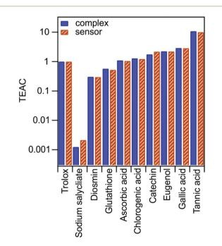
Fig. 2 TEAC values determined by Cu(Nc)<sub>2</sub> (complex) and dLDH-Alg-Cu(Nc)<sub>2</sub> (sensor) for different molecular antioxidants using eqn (4).
