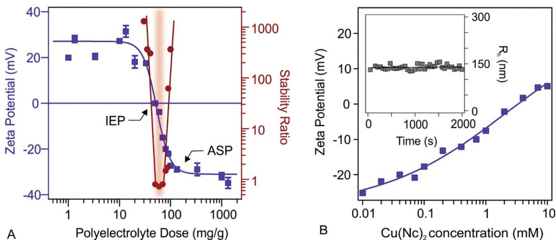
**Fig. 1** (A) Zeta potential and stability ratio values at different polyelectrolyte doses. (B) Zeta potentials as a function of the complex concentration. The inset (in B) shows the hydrodynamic radius in time at 0.1 mM Cu(Nc)<sub>2</sub> concentration. The solid lines are a guide to the eye. The polyelectrolyte dose in A refers to mg NaAlg per 1 g of dLDH.
