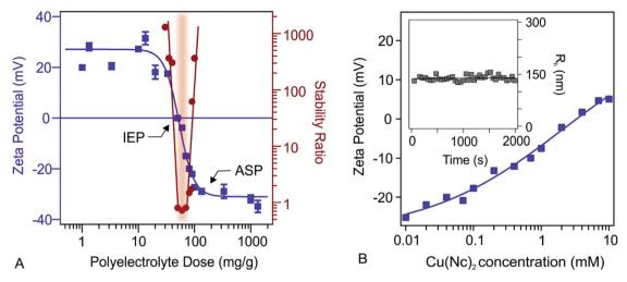
Fig. 1 (A) Zeta potential and stability ratio values at different polyelectrolyte doses. (B) Zeta potentials as a function of the complex concentration. The inset (in B) shows the hydrodynamic radius in time at 0.1 mM Cu(Nc)<sub>2</sub> concentration. The solid lines are a guide to the eye. The polyelectrolyte dose in A refers to mg NaAlq per 1 g of dLDH.
