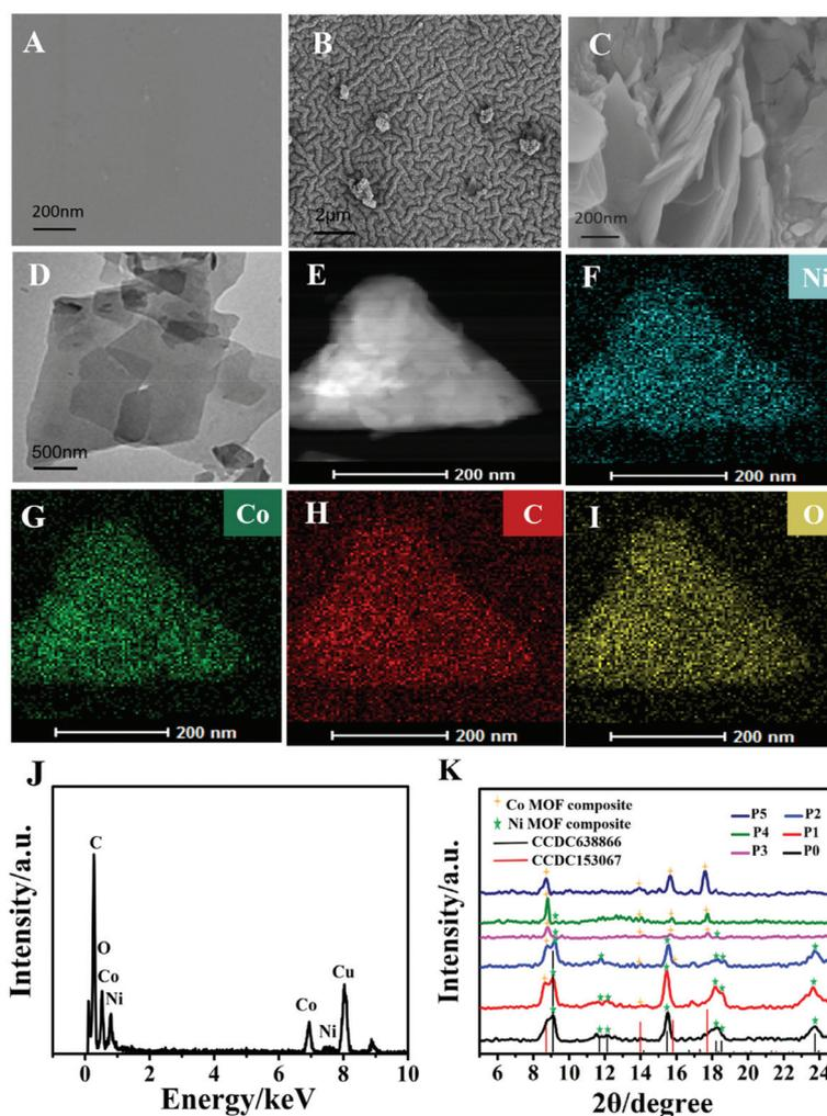
**Fig. 1** (A) SEM image of the PDMS surface. (B) SEM image of a gold layer deposited on the PDMS surface. (C) SEM image of the gold film electrode modified Ni-Co MOF (P4) nanocomposite. (D) TEM image of the Ni-Co MOF (P4) nanocomposite. (E–I) EDS-mapping images of the Ni-Co MOF nanocomposite. (J) EDX spectra of the Ni-Co MOF nanocomposite. (K) XRD pattern of the Ni-Co MOF nanocomposite synthesized at different nickel to cobalt ratios.
