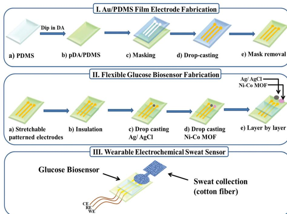
**Scheme 1** Schematic diagram of the manufacturing process of a flexible electrochemical sweat sensor based on the Ni–Co MOF nanosheet coated Au/PDMS film for glucose detection. (I) Manufacturing of flexible Au/PDMS film electrodes by a chemical deposition method. (II) Manufacturing of a flexible three-electrode system. (III) Schematic diagram of the wearable electrochemical sweat sensor.
