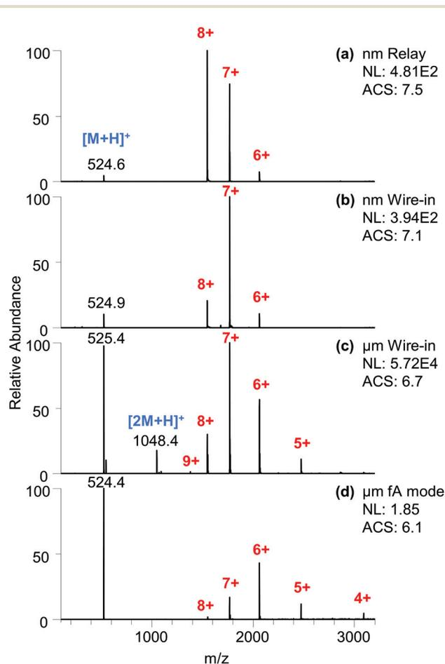
**Fig. 3** Full scan mass spectra of a 50  $\mu\text{M}$  cyt c and 50  $\mu\text{M}$  MRFA aqueous mixture under different conditions. (a) Relay ESI using a submicron emitter tip with a 7.7 pL min<sup>-1</sup> flow rate. (b) Wire-in ESI using a submicron emitter tip. (c) NanoESI using a micrometer emitter tip. (d) fA ESI using a micrometer emitter tip.
