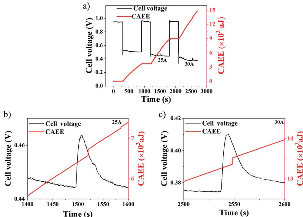
Fig. 8 (a) Voltage and CAEE variation during galvanostatic tests at 20 A ( $0.8 \text{ A cm}^{-2}$ ), 25 A ( $1 \text{ A cm}^{-2}$ ) and 30 A ( $1.2 \text{ A cm}^{-2}$ ); (b) and (c) show voltage and CAEE response for key features during the 25 A ( $1 \text{ A cm}^{-2}$ ) and 30 A ( $1.2 \text{ A cm}^{-2}$ ) hold, respectively.
