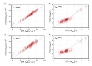
Fig. 4 Scatter plots of DFT against the predicted data with QBF and MVS inputs for  $G_{\rm rel}$  (panels a and c) and  $E_{\rm exc}$  (b and d). Error bars represent the standard deviation of the prediction, and the blue hashed line is the identity line, provided as a guide. The arrows in (a) and (c) mark the outliers, see text.
