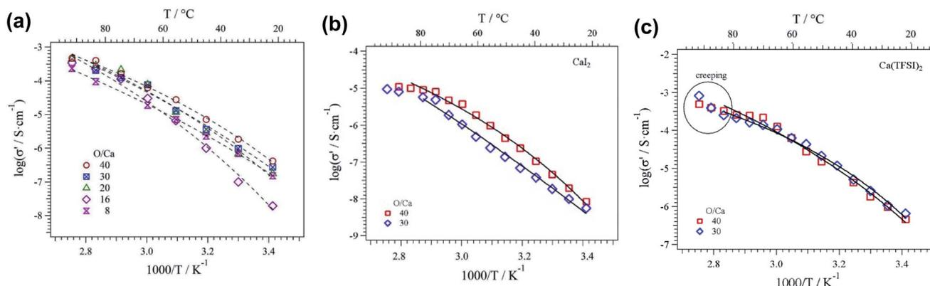
Fig. 13 Ionic conductivity as a function of temperature for POE- $\text{Ca}(\text{CF}_3\text{SO}_3)_2$  (a), POE- $\text{Ca}_2$  (b), and POE- $\text{Ca}(\text{TFSI})_2$  (c) electrolytes. Continuous lines correspond to Vogel-Tamman-Fulcher fitting. Adapted with permission from ref. 44. Copyright 2020 Elsevier.
