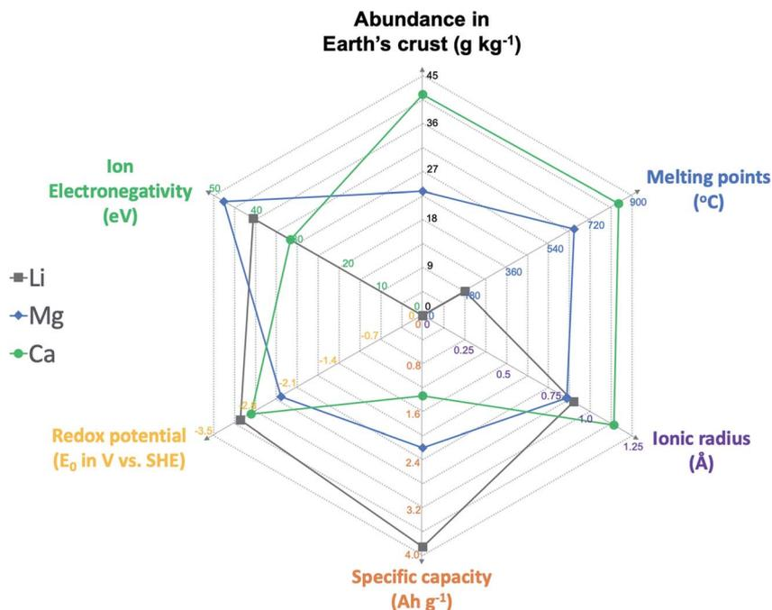
Fig. 1 Physical properties of Li, Mg, and Ca elements, including abundance in the Earth's crust ( $\text{g kg}^{-1}$ ), melting point ( $^{\circ}\text{C}$ ), ionic radius ( $\text{\AA}$ ), specific capacity ( $\text{Ah g}^{-1}$ ), redox potential (V vs. SHE), and ion electronegativity (eV).
