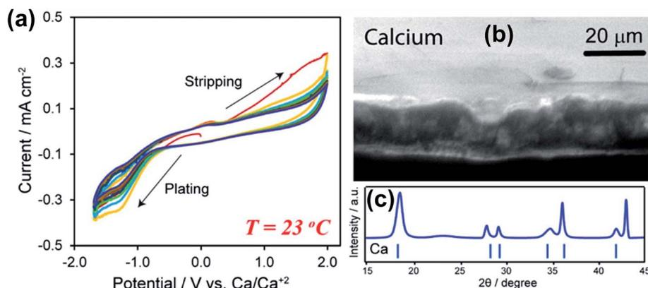
Fig. 4 Electrochemical studies of  $\text{Ca}(\text{BF}_4)_2$ -EC/PC electrolytes at room temperature. (a) Cyclic voltammograms of a 1.0 M  $\text{Ca}(\text{BF}_4)_2$  electrolyte. (b) A SEM image of deposited Ca metal. (c) XRD pattern of deposited Ca metal. Adapted with permission from ref. 24. Copyright 2019 American Chemical Society.
