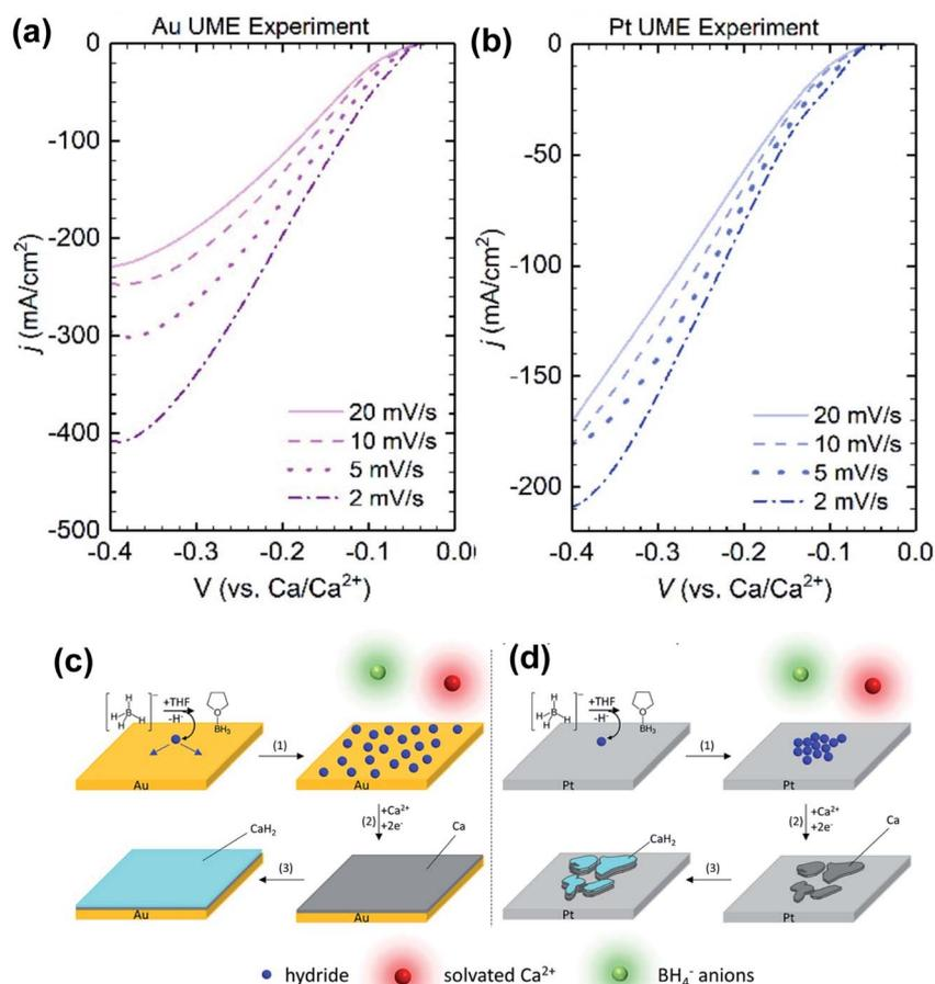
Fig. 7 Electrochemical studies of the  $\text{Ca}(\text{BH}_4)_2$ -THF electrolyte by Gewirth and co-workers. (a) and (b) Dependence of deposition current with scan rate using Au and Pt working electrodes, respectively. (c) and (d) Proposed deposition mechanisms using Au and Pt working electrodes, respectively. Adapted with permission from ref. 27. Copyright 2020 American Chemical Society.
