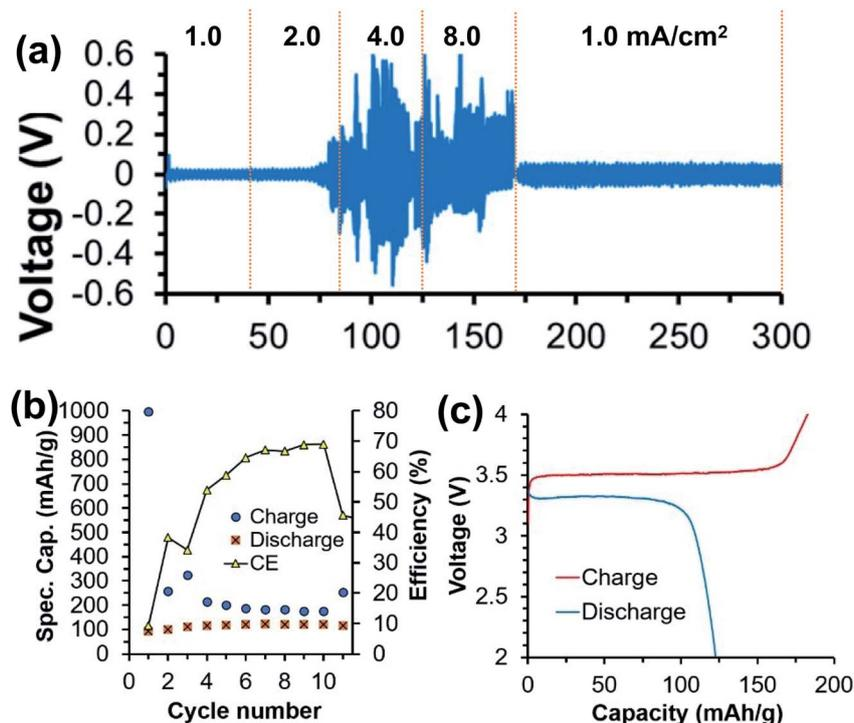
Fig. 12 Half-cell and full-cell studies of a 0.25 M  $\text{Ca}[\text{B}(\text{hfip})_4]_2$ -DGM electrolyte. (a) A  $\text{Ca}||\text{Ca}$  symmetric cell using a  $\text{Ca}[\text{B}(\text{hfip})_4]_2$ -DGM electrolyte. (b) Cycling performance and (c) representative charge/discharge profiles of a  $\text{Ca}||\text{FePO}_4$  full battery using the  $\text{Ca}[\text{B}(\text{hfip})_4]_2$ -DGM electrolyte. Adapted with permission from ref. 40. Copyright 2020 Wiley-VCH.
