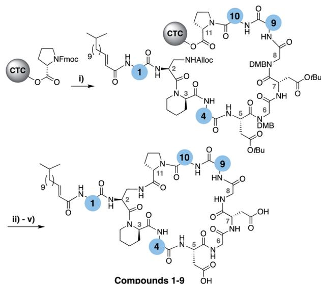
Scheme 1 (i) Fmoc SPPS; (ii) Pd(PPh<sub>3</sub>)<sub>4</sub>, PdSiH<sub>3</sub>, CH<sub>2</sub>Cl<sub>2</sub>, 1 h; (iii) HFIP, CH<sub>2</sub>Cl<sub>2</sub>, 1 h; (iv) BOP, DIPEA, CH<sub>2</sub>Cl<sub>2</sub>, 16 h; (v) TFA, TIS, H<sub>2</sub>O, 1 h.
