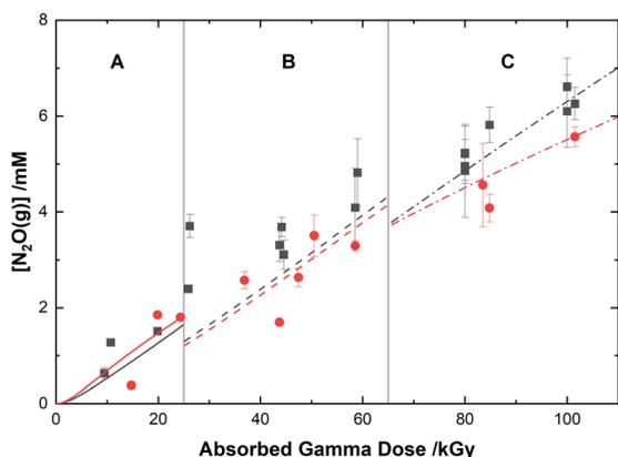
**Fig. 8** Yields of N<sub>2</sub>O from the gamma irradiation of 0.50 M AHA in water (■) and 0.20 M HClO<sub>4</sub> (●). The experimental data are divided into three regions: (A) 51 Gy min<sup>-1</sup> at 36 °C (solid curve), (B) 150 Gy min<sup>-1</sup> at 40 °C (dashed curve), and (C) 250 Gy min<sup>-1</sup> at 42 °C (dash-dot curve). Lines are predicted values from multiscale modelling calculations.
