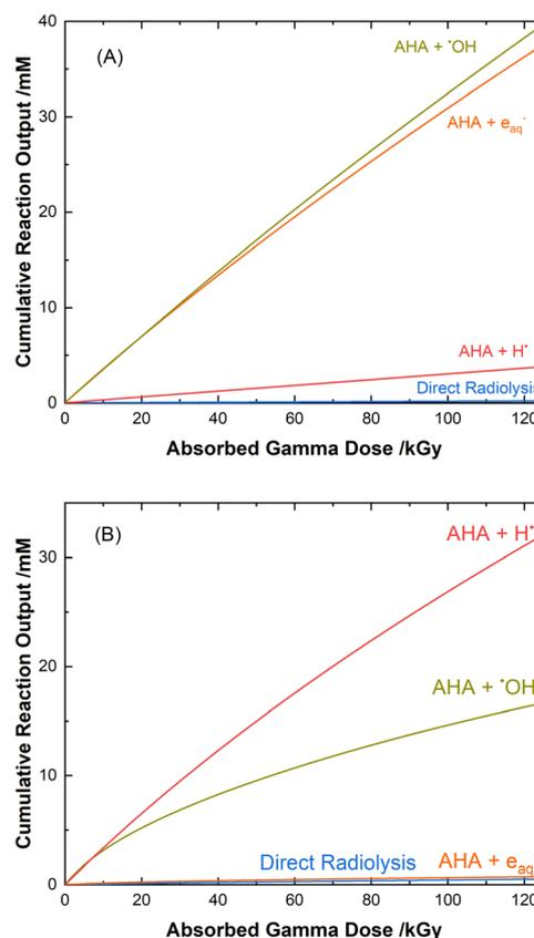
**Fig. 3** Multiscale model calculated cumulative reaction outputs for the major pathways involved in the radical-induced loss of 0.5 M AHA for  $51 \text{ Gy min}^{-1}$  at  $36^\circ\text{C}$  in (A) water and (B) 0.20 M  $\text{HClO}_4$ .
