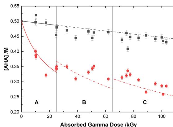
Fig. 2 Concentration of 0.50 M AHA as a function of absorbed gamma dose in water (■), and 0.20 M HClO<sub>4</sub> (●). The experimental data points are divided into three regions: (A) 51 Gy min<sup>-1</sup> at 36 °C (solid curve); (B) 150 Gy min<sup>-1</sup> at 40 °C (dashed curve); and (C) 250 Gy min<sup>-1</sup> at 42 °C (dash-dot curve). Lines are predicted values from multiscale modelling calculations.
