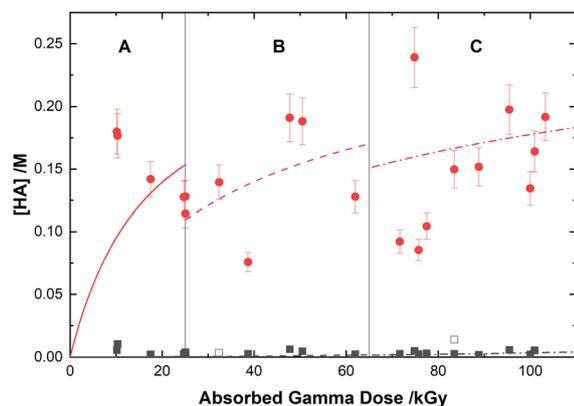
**Fig. 6** Yields of HA from the gamma irradiation of 0.50 M AHA in water (■) and 0.20 M HClO<sub>4</sub> (●). The experimental data are from UV-vis spectroscopy (filled symbols) and <sup>1</sup>H-NMR (open symbols), and are divided into three regions: (A) 51 Gy min<sup>-1</sup> at 36 °C (solid curve), (B) 150 Gy min<sup>-1</sup> at 40 °C (dashed curve), and (C) 250 Gy min<sup>-1</sup> at 42 °C (dotted curve). Lines are predicted values from multiscale modelling calculations.
