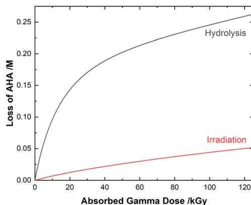
Fig. 4 Multiscale model calculated relative contributions of hydrolysis and gamma radiolysis reactions to the cumulative loss of 0.50 M AHA for 51 Gy min<sup>-1</sup> at 36 °C in 0.20 M HClO<sub>4</sub>.
