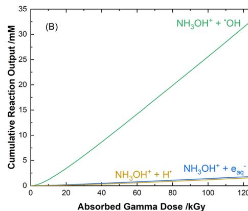
**Fig. 7** Calculated cumulative reaction yields for the major pathways involved in the radiolytic loss of HA for 51 Gy min<sup>-1</sup> gamma irradiation at 36 °C in 0.5 M AHA in (A) water, and (B) 0.20 M HClO<sub>4</sub>.
