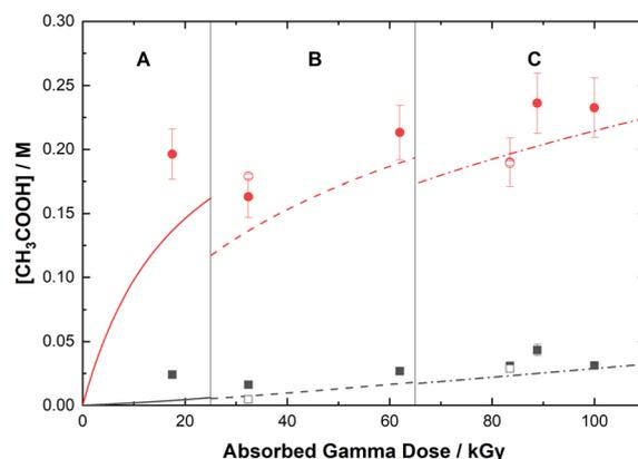
Fig. 5 Yields of acetic acid from the gamma irradiation of 0.50 M AHA in water (■) and 0.20 M HClO<sub>4</sub> (●). The experimental data are from IC (filled symbols) and <sup>1</sup>H-NMR (open symbols) and are divided into three regions: (A) 51 Gy min<sup>-1</sup> at 36 °C (solid curve), (B) 150 Gy min<sup>-1</sup> at 40 °C (dashed curve), and (C) 250 Gy min<sup>-1</sup> at 42 °C (dash-dot curve). Lines are predicted values from multiscale modelling calculations.
