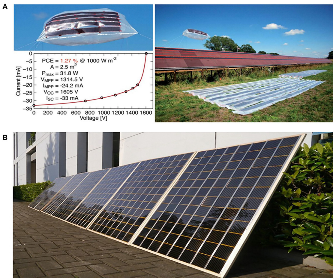
Fig. 18 Installations of OSC and PSC modules. (A) Photograph of the helium-filled balloon with attached solar cells and an I - V -curve (left). The photograph on the right shows three installation scenarios combined – balloon, wooden solar park structure (with just 2 stripes of solar cells), and tubes (flat, and blown-up in the background). Reproduced with permission from Espinosa et al. , 233 Copyright 2014 Royal Society of Chemistry. (B) Image of 7 m 2 printable perovskite solar panels. Reproduced with permission from Hu et al. , 235 Copyright 2017 Wiley-VCH GmbH.
