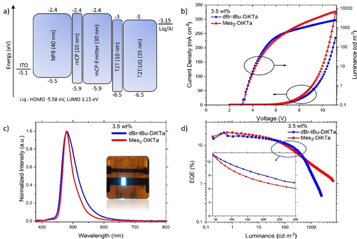
Fig. 7 OLEDs JVL results. (a) Device architecture, (b) JVL curves, (c) EL spectra and (d) EQE vs. luminance of **dBr-tBu-DiKTA** (blue) and **Mes<sub>3</sub>-DiKTA** (red). Inset in figure (d): linear EQE vs. luminance to highlight the roll-off difference in the noted region.
