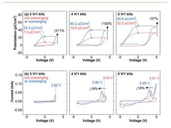
Fig. 3 (a) P-V curves by the PUND method. (b) I-V curves using a bipolar triangular pulse. The  $V_{\rm sw}$  of the capacitor with scavenging was lower than that of the capacitor without scavenging. Due to the lower  $V_{\rm sw}$ , the  $P_{\rm r}$  of the capacitor with scavenging was higher than that of the capacitor without scavenging at the same pulse amplitudes.
