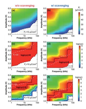
Fig. 4 Maps of  $P_r$  extracted from the PUND method of capacitors (a) without scavenging and (b) with scavenging. Endurance maps until (c), (d) breakdown occurred and (e), (f)  $P_r$  reached 10  $\mu$ C cm $^{-2}$ . The black and white dashed lines indicate  $P_r$  of 10 and 30  $\mu$ C cm $^{-2}$ , respectively. The black solid line indicates the region with endurance cycles higher than  $10^6$ .
