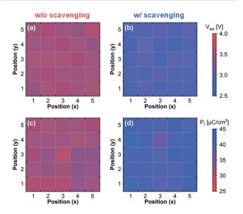
Fig. 6 Uniformity maps of (a), (b)  $V_{\rm sw}$  and (c), (d)  $P_{\rm r}$  of capacitors without and with scavenging. 25 capacitors for each were measured in an area of  $1\times 1~{\rm cm}^2$ .
