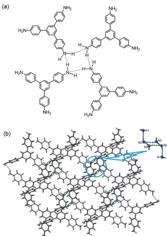
Fig. 2 Supramolecular structure of **1**, (a) depiction of intermolecular N-H...N hydrogen bonds (red dotted bonds) and (b) crystal structure (inset shows a cluster of six -NH<sub>2</sub> groups, connected by hydrogen bonds). Reproduced from ref. 40 with permission. Copyright© 2014, American Chemical Society.
