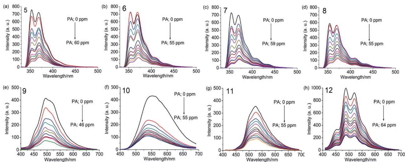
**Fig. 7** Photoluminescence spectra of 5–8 in dichloromethane ( $1.0 \times 10^{-6}$  M,  $\lambda_{\text{ex}} = 295$  nm) and 9–12 in acetonitrile ( $0.2$  mg mL<sup>-1</sup>,  $\lambda_{\text{ex}} = 300$  nm), with progressive additions of PA. Reproduced from ref. 43 with permission. Copyright© 2016, Wiley-VCH Verlag GmbH & Co. KGaA, Weinheim.
