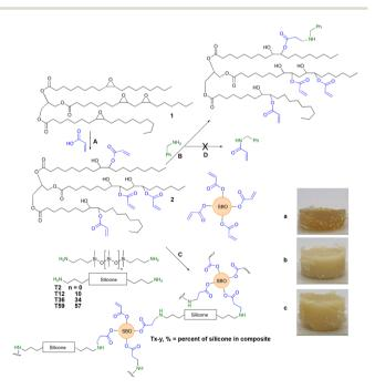
Fig. 1 (A) Formation of soybean acrylates from the epoxide; (B) Model aza-Michael reaction with benzylamine (Fig. S1, ESI†); and (C) crosslinked soybean silicones following the aza-Michael reaction between acrylated soybean oil and telechelic silicones. Photos of elastomers formed from different aminosilicones (a) T12-25, (b) T36-25 and (c) T59-25. Note: although the soybean oil sample had 4.2 alkenes per molecule, only 4 alkenes are drawn for clarity.
