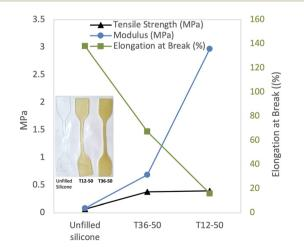
Fig. 3 Comparison of % elongation at break of: unfilled silicone, T36-50 and T12-50. Note: the lines are only to facilitate reading the chart.
