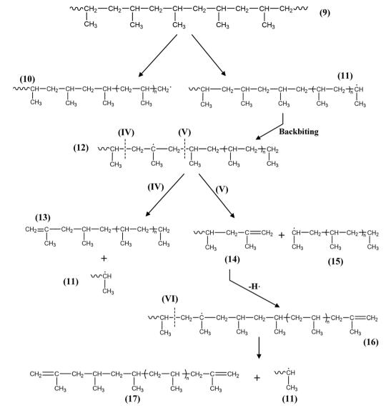
Scheme 2 Fundamental reactions for the thermal decomposition of PP leading to alkenes and alkadienes. Arabic numerals indicate chemical species that form during the pyrolysis of PE, while Roman numerals indicate the occurrence and position of the scission of a chemical bond.
