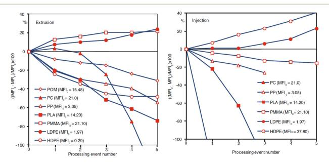
Fig. 12 Change in MFI as a function of number of processing events for extrusion (left) and injection molding (right). MFI<sub>0</sub> and MFI<sub>F</sub> are the MFI prior to any processing event and the MFI after the total processing events, respectively. Published from ref. 32 with permission from Carl Hanser Verlag, Munich, copyright 2012.
