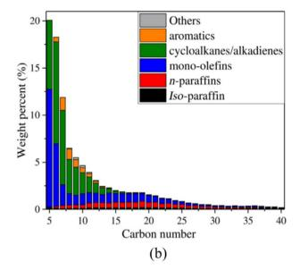
Fig. 17 (a) A typical naphtha composition (graph made based on the data obtained from ref. 251, (b) a typical plastic pyrolysis oil composition obtained from PE pyrolysis. Reproduced from ref. 252 with permission from Wiley-VCH, copyright 2020.
