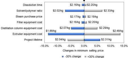
Fig. 25 Sensitivity analysis of MSP for the STRAP process. Reproduced from ref. 609 with permission from Wiley-VCH, copyright 2021.
