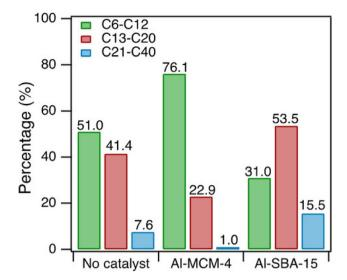
Fig. 20 Distribution of liquid and wax products for thermal pyrolysis and mesoporous aluminosilicates in the conversion of PE/PP (ratio 6:5). Pyrolysis experiments were conducted at 500 °C for 30 minutes using a batch reactor set up, where the catalyst-to-feedstock ratio was 0.03:1. Reproduced from ref. 401 with permission from Wiley-VCH, copyright 2020.
