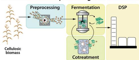
Fig. 7 Flow sheets comparing the Base Case (A) and Advanced Scenario (B) from Lynd *et al.* (2017). "DSP" denotes downstream processing and separation. Carbohydrate-active enzymes are produced aerobically in a dedicated unit operation for (A), but are produced during fermentation by an anaerobic, biofuel-producing culture for (B).
