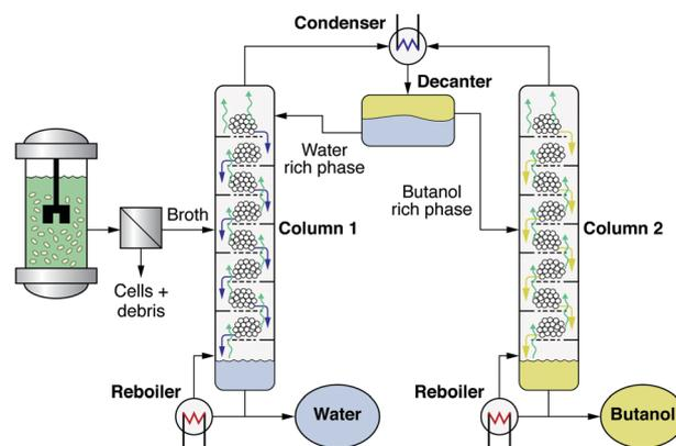
Fig. 9 Illustration of heteroazeotropic distillation for the separation of butanols from fermentation broth. A detailed set of operation parameters for these columns can be found in Luyben, 2008.<sup>210</sup>
