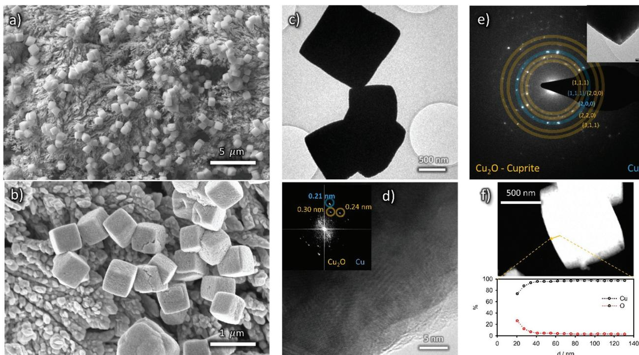
**Fig. 1** (a and b) FE-SEM images of bare OD-Cu; (c) low magnification and (d) HR-TEM micrographs of OD-Cu nanocubes displaying reflections compatible with  $\text{Cu}_2\text{O}$  and the Cu lattice (FFT in figure d inset); (e) selected area electron diffraction (SAED) of a single nanocube (inset) highlighting concurrent cuprite and metallic Cu phases; (f) STEM-HAADF micrograph of a single cube and Cu/O content obtained by EDS analysis along the highlighted profile.
