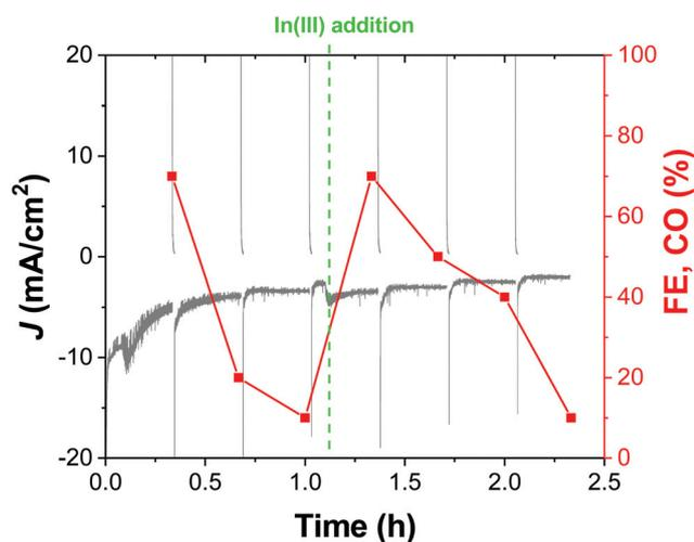
**Fig. 8** Chronoamperometric trace of the OD-Cu\_In36 cathode stepped between -0.72 V and the open circuit potential, OCP. The faradaic efficiency for CO production at different sampling times is also reported. The green dashed line marks the addition of 1 mL of a 0.04 M solution of In(NO<sub>3</sub>)<sub>3</sub> in 0.5 M citric acid, aimed at restoring the active In-based layer and consequently the previous CO production.
