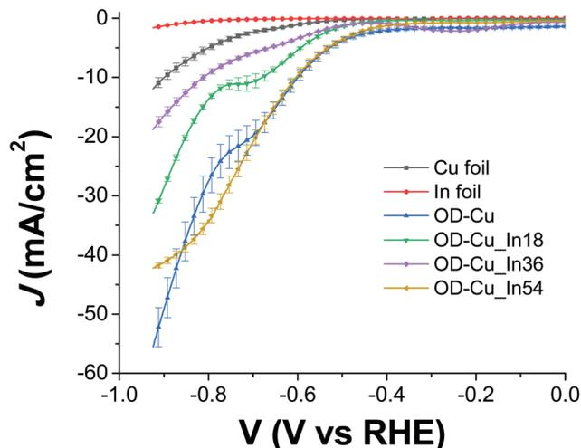
**Fig. 6**  $J$ - $V$  characteristics for the tested cathodes, recorded in 0.5 M  $\text{KHCO}_3$  saturated with  $\text{CO}_2$  (pH 7.4), normalized for the geometric area and corrected for the iR drop. The stable response of at least three electrodes has been averaged, and the corresponding curves are reported, together with the error bars.
