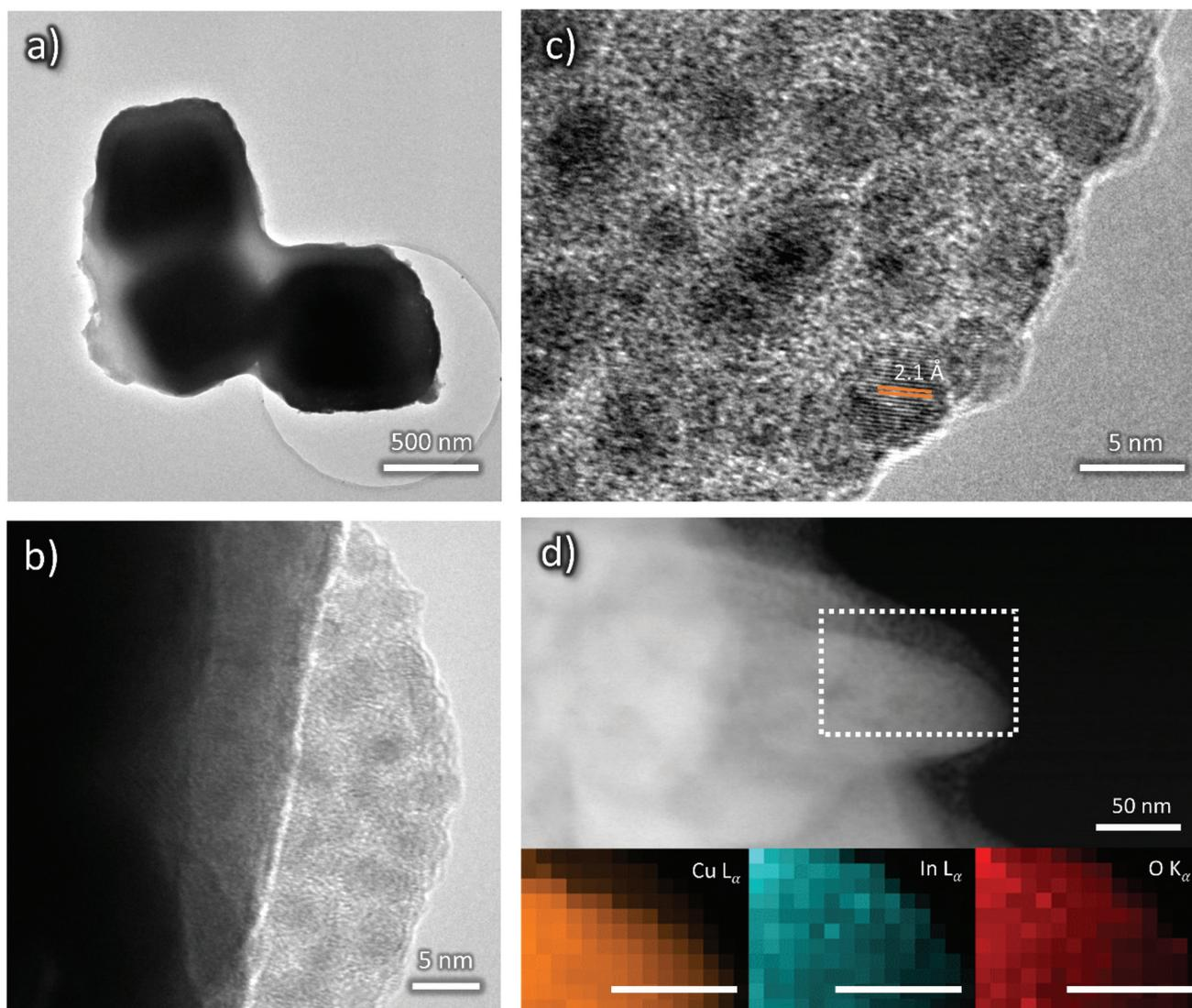
**Fig. 4** (a) Low magnification TEM and (b and c) HR-TEM micrographs of the OD-Cu<sub>In</sub>18 sample. The coating layer around the Cu nanocubes embeds the crystalline nanoparticles, the *d*-spacing of which is compatible with that of In<sub>2</sub>O<sub>3</sub> or In(OH)<sub>3</sub>. (d) STEM-HAADF micrograph of an OD-Cu<sub>In</sub>18 nanocube surface feature and related EDS mapping displaying higher concentrations of In and O in the coating layer.
