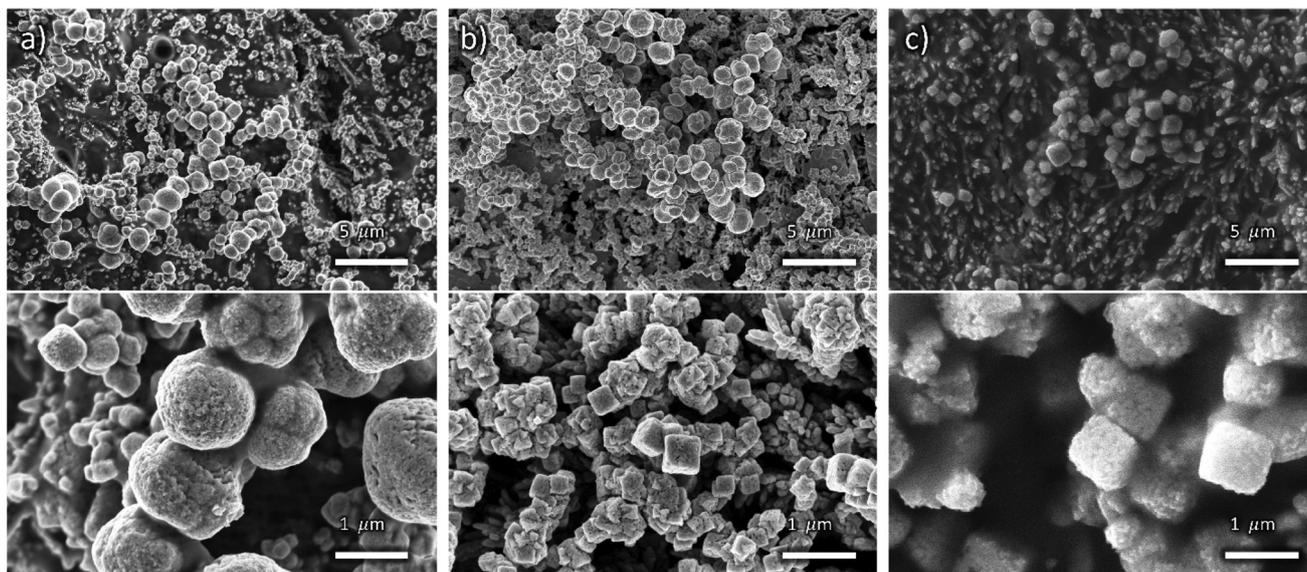
Fig. 3 Low (top) and high (bottom) magnification FE-SEM images of OD-Cu<sub>In</sub>18 (a), OD-Cu<sub>In</sub>36 (b) and OD-Cu<sub>In</sub>54 (c).
