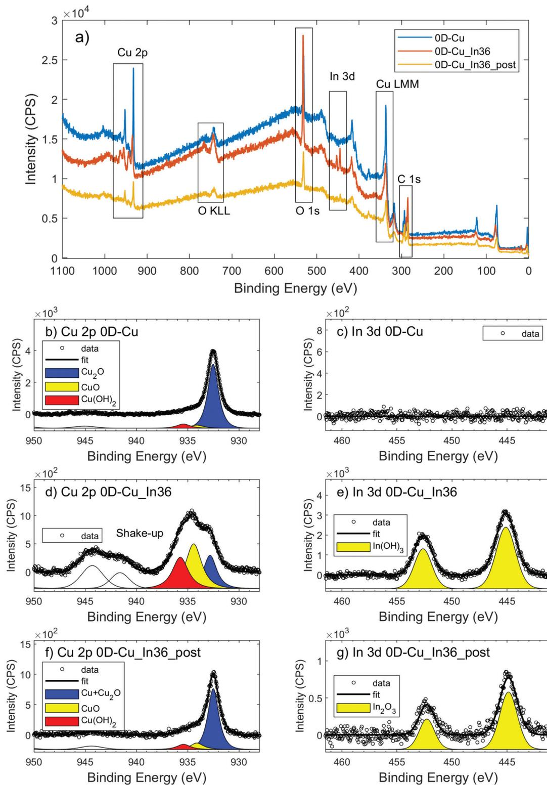
**Fig. 5** (a) Survey XPS spectra of OD-Cu (blue), OD-Cu\_In36 (red) and OD-Cu\_In36\_post (orange). XPS signals of Cu 2p, O 1s, In 3d, C 1s and K 2p are present, with Auger signals of O KLL and Cu LMM; (b-d-f) high resolution spectra of Cu 2p<sub>3/2</sub> in OD-Cu (b), OD-Cu\_In36 (d) and OD-Cu\_In36\_post (f); (c-e-g) high resolution spectra of In 3d in OD-Cu (c), OD-Cu\_In36 (e) and OD-Cu\_In36\_post (g).
