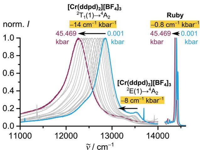
Fig. 7 Normalized pressure-dependent phosphorescence spectra of  $[\text{Cr}(\text{ddpd})_2][\text{BF}_4]_3$  between 0.001 and 45.469 kbar in nujol together with a ruby crystal (right).<sup>20,23</sup>
