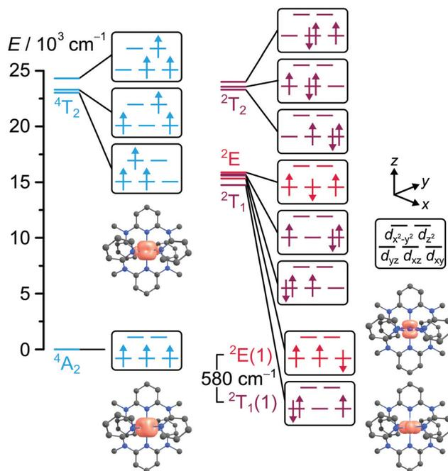
Fig. 4 CASSCF(7,12)-NEVPT2 derived state diagram at the GS geometry of  $[\text{Cr}(\text{ddpd})_2]^{3+}$  with dominating electron configurations in the micro-states and calculated spin-densities at an isosurface value of 0.05 a.u.<sup>20</sup>
