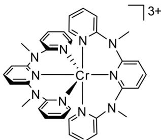
Fig. 2 Molecular structure of  $[\text{Cr}(\text{ddpd})_2]^{3+}$ .
