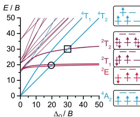
**Fig. 1** Tanabe–Sugano (TS) diagram of the *d*<sup>3</sup> electron configuration in an octahedral ligand field with *C/B* = 4 and exemplary microstates.<sup>4,14</sup> The two important excited state quartet/doublet crossing points are highlighted with a circle and a square, respectively. Dotted lines in the microstates indicate strong electronic mixing.
