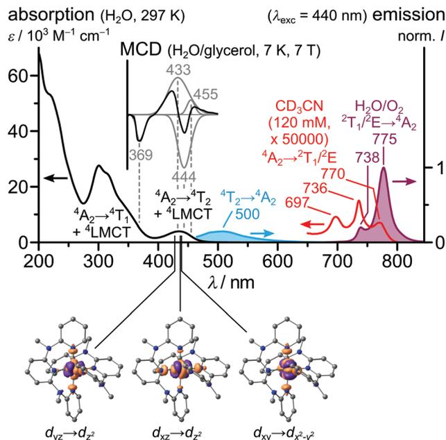
Fig. 3 Absorption spectra ( $\text{H}_2\text{O}$ : black line,  $\text{CD}_3\text{CN}$ : red line, see ESI†), MCD spectrum ( $\text{H}_2\text{O}/\text{glycerol}$ , 7 K, 7 T) and separately normalized fluorescence (blue area) and phosphorescence spectra (purple area, aerated  $\text{H}_2\text{O}$ ) of  $[\text{Cr}(\text{ddpd})_2]^{3+}$  and TD-DFT (B3LYP/Def2-TZVPP) calculated difference densities of the  $^4A_2 \rightarrow ^4T_2$  transitions with an isosurface value of 0.005 a.u.<sup>7,17</sup>
