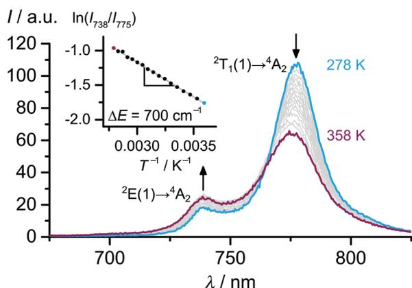
Fig. 5 Phosphorescence spectra of  $[Cr(\text{ddpd})_2][\text{BF}_4]_3$  in  $\text{H}_2\text{O}$  at variable temperature. The inset shows the Boltzmann plot  $\ln(I_{738}/I_{775})$  vs.  $T^{-1}/\text{K}^{-1}$ . The slope corresponds to  $-\Delta E/k_B$  with the energy difference of the emissive states  $\Delta E$  and the Boltzmann constant  $k_B$ .<sup>21</sup>
