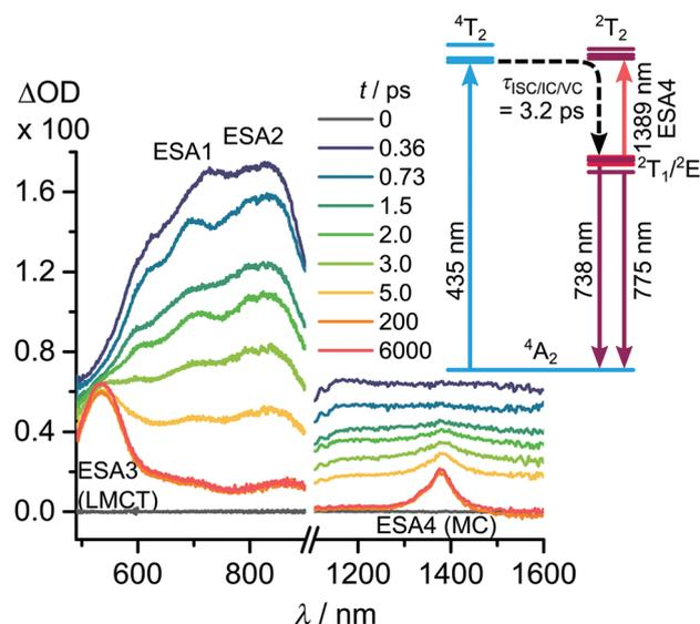
Fig. 8 Fs-Transient absorption spectra of  $[\text{Cr}(\text{ddpd})_2]^{3+}$  in  $\text{CH}_3\text{CN}$  after excitation at 435 nm and excited state diagram with CASSCF(7,12)-NEVPT2 calculated energies (see ESI† for details, ESA = excited state absorption).<sup>26</sup>
