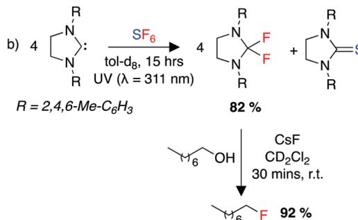
**Scheme 8** (a) Activation of  $SF_6$  by a Pt(0) complex and use of the product in a subsequent deoxyfluorination of a ketone, (b) photolytic activation of  $SF_6$  using an NHC, and subsequent deoxyfluorination of an alcohol.
