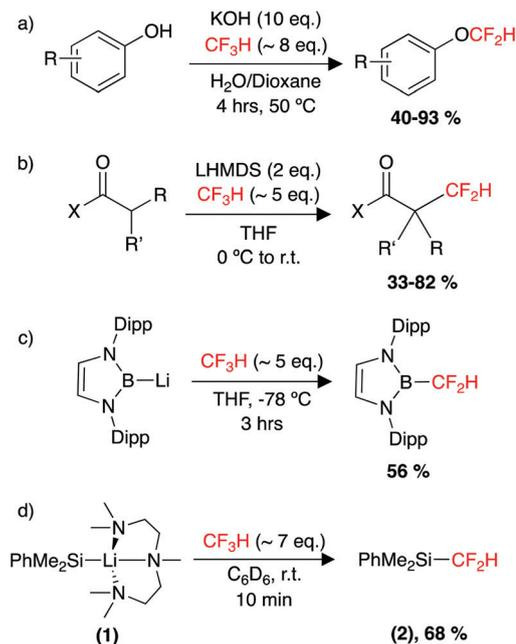
**Scheme 2** Utility of  $\text{HCF}_3$  as a feedstock, (a) in the synthesis of aryldifluoromethylethers, (b) in the  $\alpha$ -difluoromethylation of carbonyls, (c) defluoroborylation to form an organoboron building block and (d) defluorosilylation to form an organosilicon building block.
