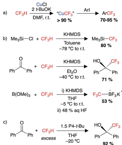
**Scheme 1** (a) Cupration of  $\text{CF}_3\text{H}$  and trifluoromethylation of aryl iodides, (b) nucleophilic trifluoromethylation of a range of electrophiles using  $\text{CF}_3\text{H}$  as a feedstock. HMDS = hexamethyldisilazane, (c) trifluoromethylation of carbonyl substrates (benzophenone shown) using  $\text{HCF}_3$  and P4-*t*-Bu superbase. P4-*t*-Bu =  $((\text{NMe}_2)_3\text{P}=\text{N})_3\text{P}=\text{N}(t\text{-Bu})$ .
