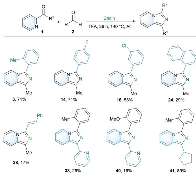
**Scheme 4** Direct utilization of chitin for the synthesis of imidazo[1,5-*a*]pyridines.  $^2\text{H}$ Pyridine ketones, aldehydes and chitin in  $\text{CF}_3\text{COOH}$  were stirred at  $140^\circ\text{C}$  under an Ar atmosphere for 36 h. Yields are those of the isolated products.
