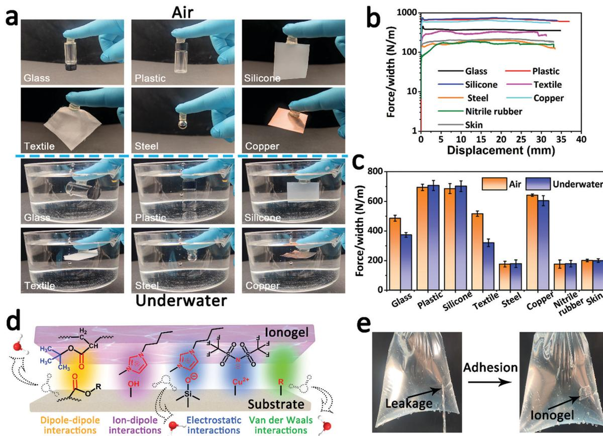
**Fig. 3** Adhesive performance of the fully hydrophobic ionogel. (a) Adhesive behavior of the ionogel with various substrates in air/under water. (b) Peeling curves of the ionogel with various substrates under water. (c) Adhesion strength of the ionogel with various substrates in air/under water. (d) Adhesion mechanisms between the ionogel and the substrate. (e) Digital images of mending a hole.
