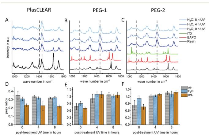
Fig. 4 Results of Raman spectroscopy on printed parts depending on the post-treatment. Fingerprint region spectra of PlasCLEAR resin (A), PEG-1 (B) and PEG-2 (C) with marked peaks used to calculate peak ratios. Peak ratios as degree of cross-linking are given for peaks at  $1410:1470 \text{ cm}^{-1}$  for PlasCLEAR (D) and at 1130: 1470 cm<sup>-1</sup> for PEG-1 (E) and PEG-2 (F).
