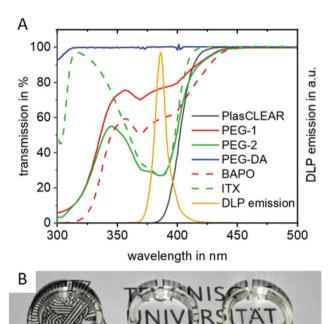
Fig. 2 UV/VIS photospectroscopy of all resins and their single components shows the transmission of light at wavelengths between 300 and 500 nm (left y-axis), with the printer's DLP emission spectrum (right v-axis) showing a clear peak at 385 nm (A). Images of printed cell culture dishes of all printing materials show the high post-printing transparency for all three selected resins (B).
