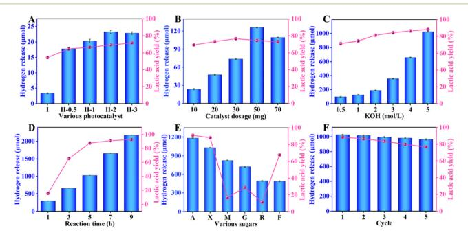
Fig. 4 The effects of various conditions on co-production of hydrogen and lactic acid, (A) different photocatalysts (I: CN, II: RuS<sub>2</sub>@CN), (B) catalyst dosages (5.0 h, 30 °C), (C) KOH concentrations (10.0 mg RuS<sub>2</sub>@CN-2, 5.0 h), (D) irradiation time (10 mg RuS<sub>2</sub>@CN-2, 5.0 M KOH). (E) The selective oxidation of different biomass-derived sugars to hydrogen and lactic acid photocatalyzed by RuS<sub>2</sub>@CN-2. (F) Recycling test of RuS<sub>2</sub>@CN-2.
