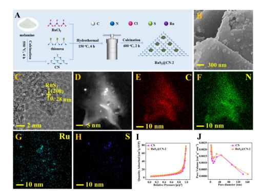
Fig. 1 Preparation scheme of  $RuS_2@CN-x$  (A). SEM image (B) and TEM images (C and D) of  $RuS_2@CN-2$ . Elemental mapping images of  $RuS_2@CN-2$ : C (E), N (F), Ru (G), S (H).  $N_2$  adsorption—desorption isotherms of CN and  $RuS_2@CN-2$  (J). Pore width distribution of CN and  $RuS_2@CN-2$  (J).
