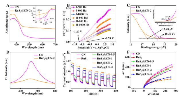
Fig. 3 UV-vis DRS of CN and RuS2@CN-2 (A). Mott-Schottky plots of CN (I) and RuS2@CN-2 (II) at frequencies of 500, 800, 1000 Hz in 0.5 M Na<sub>2</sub>SO<sub>4</sub> (B). UPS of CN and RuS<sub>2</sub>@CN-2 (C). PL of CN and RuS<sub>2</sub>@CN-2 (D). Periodic ON/OFF photocurrent responses of as-prepared samples in 0.5 M Na<sub>2</sub>SO<sub>4</sub> electrolyte under visible light irradiation ( $\lambda$  > 420 nm) at 0.5 V vs. Ag/AgCl electrode (E). EIS of as-prepared samples (F).
