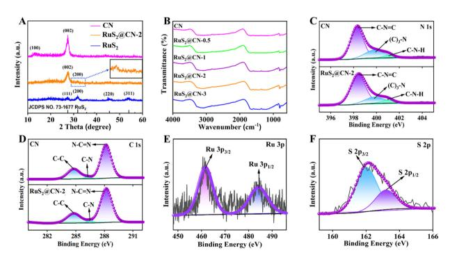
Fig. 2 XRD patterns of CN, RuS2@CN-2, and RuS2 (A). FT-IR spectra of as-prepared samples (B). XPS high-resolution spectra of CN and RuS2@CN-2: N 1s (C), C 1s (D), Ru 3p (E) and S 2p (F).
