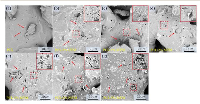
Fig. 11 After immersing in PBS for 4 weeks, the surface morphology of PCL and composite scaffolds was observed (a-g). Scaffolds with lower MTM content only show a few small pores on the surface, while PCL/3% MTM, PCL/4% MTM, and PCL/5% MTM scaffolds exhibit large areas of pore formation and collapse within the field of view. This makes it easier for the solution to penetrate the interior and promote degradation.
