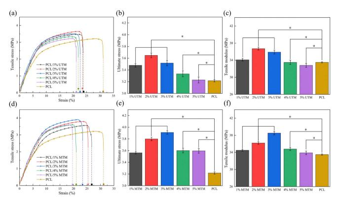
Fig. 5 (a) PCL/UTM samples tensile stress-strain curve; (b) ultimate stress and (c) tensile modulus of UTM sample; (d) PCL/MTM samples tensile stress-strain curve; (e) ultimate stress and (f) tensile modulus of MTM sample. \* Represents statistical difference (\*p < 0.05, \*\*p < 0.01 when compared with the PCL scaffold).
