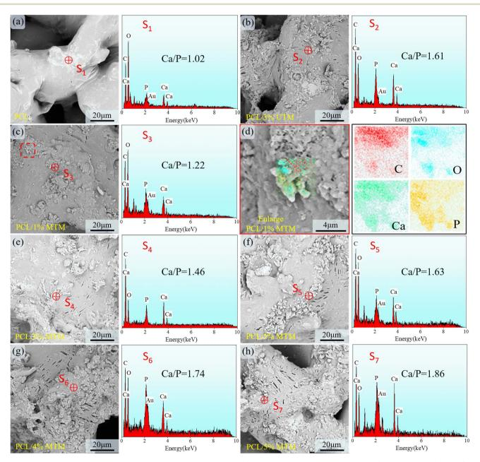
Fig. 12 SEM micrographs of the scaffolds incubated in SBF solution for 28 days and corresponding EDS spectra (magnification ×2000). (a) The PCL scaffold, (b) the PCL/3% UTM scaffold, (c) the PCL/1% MTM scaffold, (d) local face sweep of PCL/1% MTM scaffold, (e) the PCL/2% MTM scaffold, (f) the PCL/3% MTM scaffold, (g) the PCL/4% MTM scaffold, (h) the PCL/5% MTM scaffold.
