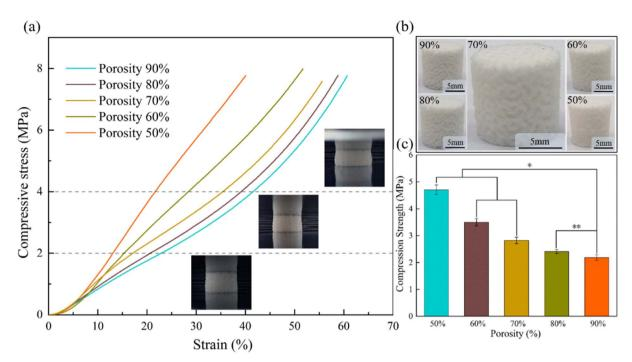
Fig. 4 (a) Comparison of compression performance of different porosity; (b) macroscopic surface morphology of pure PCL scaffolds with varying porosities; (c) stress magnitude at 25% strain. \* Represents statistical difference (\*p < 0.05, \*\*p < 0.01 when compared with the PCL scaffold with a porosity of 90%).
