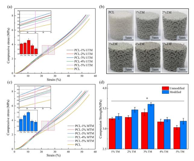
Fig. 6 (a) PCL/UTM scaffold compression stress-strain curve; (b) composite scaffold with a porosity of 70%; (c) PCL/MTM scaffold compression stress-strain curve; (d) comparison of compression stress before and after TM modification at 25% strain. \* Represents statistical difference (\*p < 0.05, \*\*p < 0.01 when compared with the PCL scaffold).
