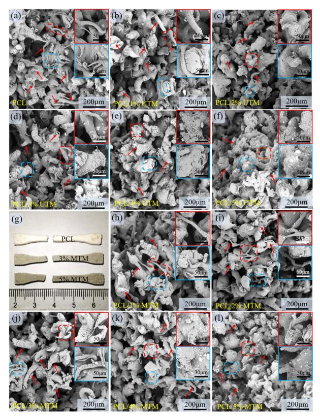
Fig. 8 SEM micrographs of the cross-sections of the tensile samples at various content (a–l). This figure provides a visual comparison showing the transformation of elongated ligaments into shorter and thicker ligaments as the TM content increases. However, when the TM content exceeds 3%, there is evidence of agglomeration at the fracture site, accompanied by detachment and the formation of voids. This leads to stress concentration, resulting in a decrease in tensile stress.
