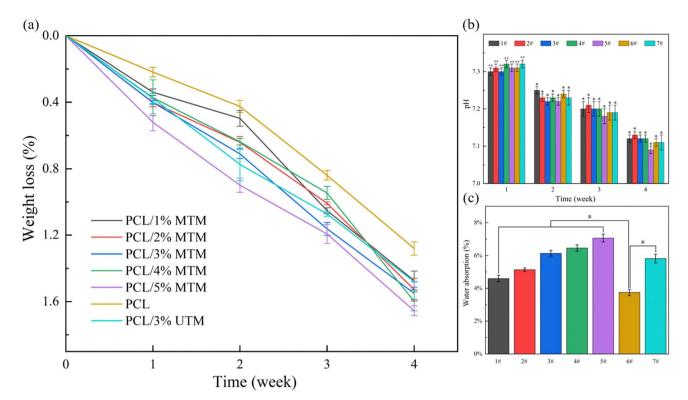
Fig. 10 (a) Weight loss of the scaffolds; (b) pH of the solution; (c) water absorption. 1# represent the PCL/1% MTM scaffold, 2# represent the PCL/ 2% MTM scaffold, 3# represents the PCL/3% MTM scaffold, 4# represents the PCL/4% MTM scaffold, 5# represents the PCL/5% MTM scaffold, 6# represents the PCL scaffold, 7# represents the PCL/3% UTM scaffold. \* Represents statistical difference (\*p < 0.05, \*\*p < 0.01 when compared with the PCL scaffold).
