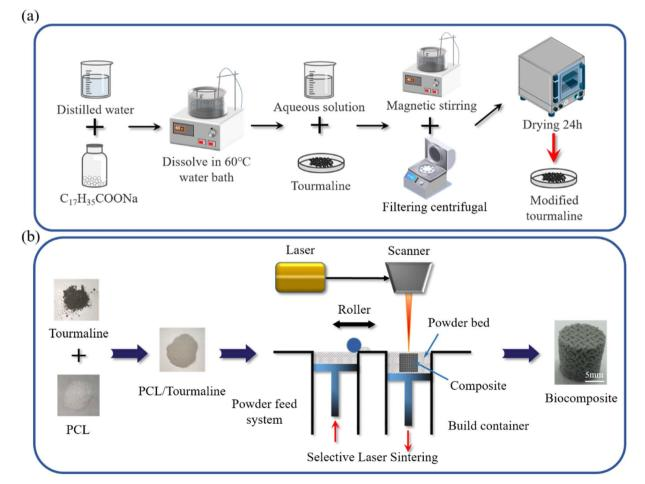
Fig. 2 (a) Schematic diagram of MTM preparation; (b) PCL/TM scaffolds with different contents were prepared by selective laser sintering.
