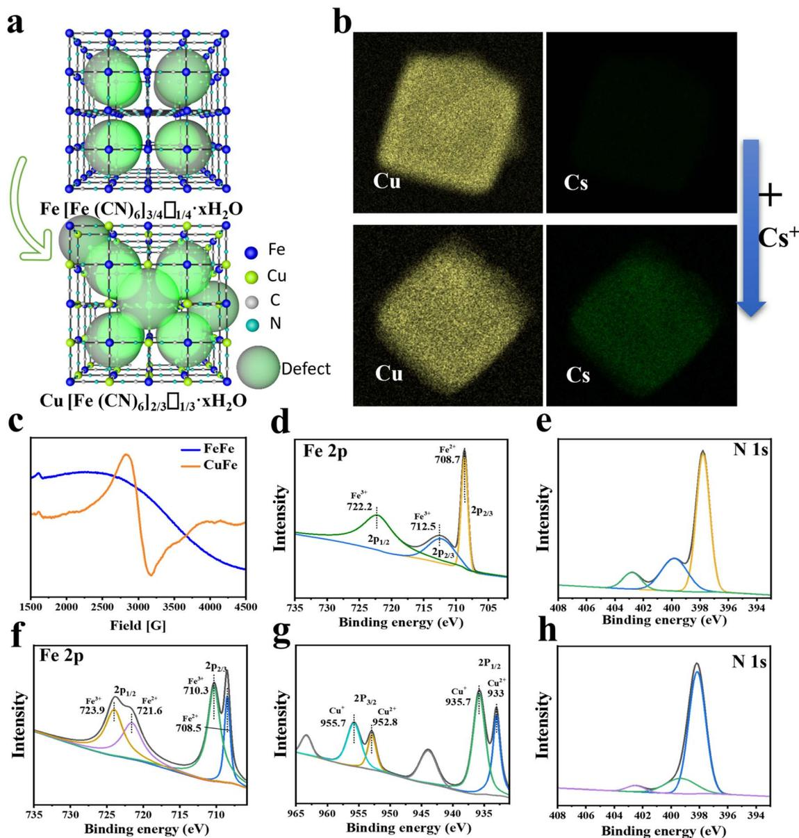
Fig. 2 (a) Schematic illustration of the defect in FeFe and CuFe. One-quarter of the  $[\text{Fe}(\text{CN})_6]$  linker is missing, generating defects (green spheres) in FeFe, and one-third of the  $[\text{Fe}(\text{CN})_6]$  linker is missing in CuFe. (b) TEM mapping of CuFe before and after the uptake of the Cs ion. (c) EPR spectra of FeFe and CuFe. (d and e), Fe 2p (d) and N 1s (e) XPS spectra of FeFe. (f–h) Fe 2p (f), Cu 2p (g) and N 1s (h) XPS spectra of CuFe.
