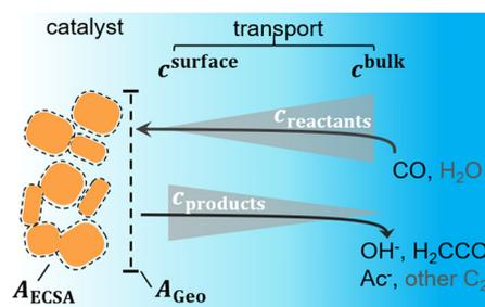
Fig. 3 Schematic of the mass transport considered in our model.  $\text{CO}$ ,  $\text{OH}^-$ ,  $\text{H}_2\text{CCO}$ , and Acetate ( $\text{Ac}^-$ ) (black color) are considered for transport while  $\text{H}_2\text{O}$  and other  $\text{C}_2$  are neglected (grey color). Typical concentration gradients are depicted and it is indicated how the transport scales with geometric area  $A_{\text{Geo}}$  while processes on the catalyst surface scale with  $A_{\text{ECSA}}$ .
