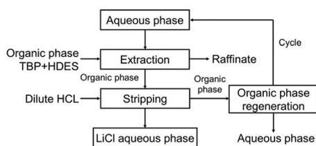
Fig. 14 Flow diagram of the TBAC : oleic acid DES-based system from Li recovery process from the mother liquor obtained during the production of  $\text{Li}_2\text{CO}_3$ . Reprint with permission from ref. 128, Copyright © 2021, Elsevier B.V.
