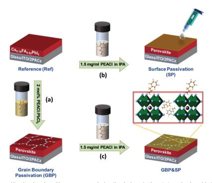
Fig. 1 Schematic of the perovskite absorber deposition process employing the dual passivation strategy developed in this work: (a) grain boundary passivation (GBP) by incorporation of PEACl:PbCl2 into the perovskite precursor solution, (b) surface passivation (SP) by treatment of PEACl in IPA on top of the perovskite absorber layer and (c) combination of grain boundary and surface passivation (GBP&SP)
