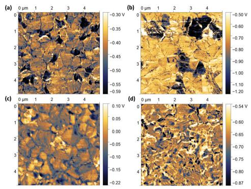
Fig. 6 Kelvin pobe force microscopy (KPFM) images for perovskite films with the structure ITO/2PACz/perovskite/ $C_{60}$  prepared (a) without any modification (Ref), (b) with grain boundary passivation (GBP), (c) surface passivation (SP), and (d) grain boundary & surface passivation (GBP&SP) processes
