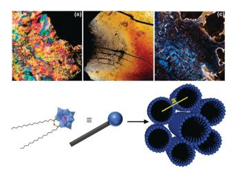
Fig. 19 Top: Polarisation microscopy images of (a) Na<sub>3</sub>[PW<sub>11</sub>O<sub>39</sub>(SiC<sub>12</sub>H<sub>25</sub>)<sub>2</sub>O], (b)  $Na_3[PW_{11}O_{39}(SiC_{16}H_{33})_2O]$  and (c)  $(TBA)_3[PW_{11}O_{39}(SiC_{16}H_{33})_2O]$ . Bottom: Schematic representation of the  $[PW_{11}O_{39}(SiC_{16}H_{33})_2O]^{3-}$  structure. This figure has been adapted from ref. 119 with permission from the American Chemical Society, Copyright 2010
