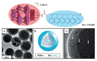
Fig. 11 (Top) Molecular structure of a POM-polystyrene hybrid; (bottom) representations of its vesicular aggregates, showing: (a,c) high-resolution TEM images and, (b) a schematic representation of the vesicle. This figure has been adapted from ref. 114 with permission from John Wiley and Sons, copyright 2012.
