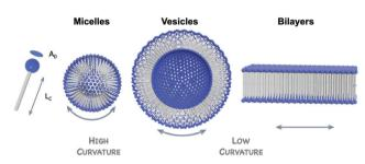
Fig. 10 Schematic highlighting the common structures of amphiphilic hybrid-POM supramolecular assemblies, which depend on both the shape of the POM-surfactant and the packing parameter (defined as  $P = V/(A_0L_C)$ ), where V represents the volume occupied by the hydrophobic tails,  $A_0$  the area of the polar head and  $L_{\mathbb{C}}$  the length of the hydrophobic tails).
