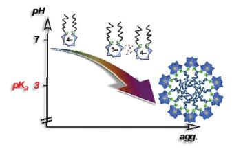
Fig. 13 Schematic showing aggregation as a function of the pH in a 10 mM agueous solution of  $K_3H[\gamma-SiW_{10}O_{36}(POC_{12}H_{25})_2]$  (> CMC). 122
