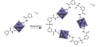
Fig. 4 Synthesis of a POM-based trimer from a bis(pyridine-trisalkoxo)hexavanadate anion and trans-[PdCl<sub>2</sub>(CH<sub>3</sub>CN)<sub>2</sub>]. This figure has been adapted from ref. 80 with permission from the Royal Society of Chemistry, copyright 2012.
