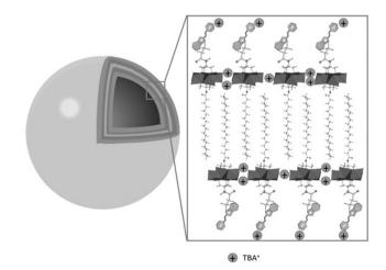
Fig. 16 Self-assembly of the photoswitchable asymmetric POM hybrid, SP-POM-C16 (SP = spiropyran, C16 = decahexane) in polar solvents to form hollow vesicles. This figure has been adapted from ref. 141 with permission from John Wiley and Sons, copyright 2016.
