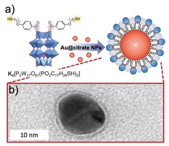
Fig. 18 (a) Structure of the thiolated hybrid POM,  $K_6[P_2W_{17}O_{61}]$ {PO<sub>2</sub>C<sub>17</sub>H<sub>26</sub>SH}<sub>2</sub>], showing its spontaneous exchange with citrate to produce covalently functionalised Au nanoparticles; (b) HR-TEM micrograph of a single Au@POM nanoparticle. This figure has been adapted from ref. 162 under the Creative Commons CC BY License.
