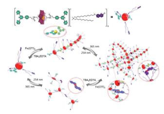
Fig. 2 Schematic illustration of the elaboration of supramolecular polymer *via* orthogonal self-assembly strategy combining metal coordination and photocross-linking. This figure has been adapted from ref. 70 with permission from the American Chemical Society, copyright 2019.
