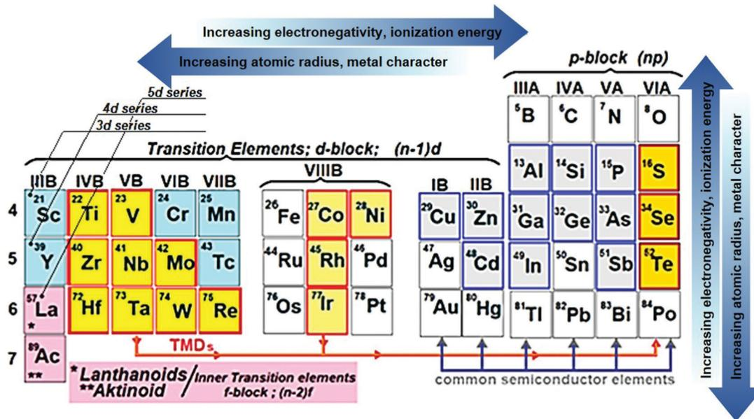
Fig. 2 Selected elements across the periodic table that—as a single element (e.g., Si, Ge), compounds (e.g., GaAs, CdAs), or alloys (e.g.,  $\text{Si}_x\text{Ge}_{1-x}$ ,  $\text{Al}_x\text{Ga}_{1-x}$ )—display semiconductor nature (into the blue frame) and the transition metals and three chalcogen (X) elements (enclosed by a red frame) that predominantly crystallize in layered TMDs. Partial highlights for Co, Rd, Ir, and Ni indicate that only some of their TMDs form layered structures.
