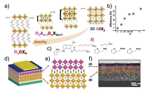
Fig. 25 (a) Structure of perovskite from 2D to 3D forms. (b)  $\eta$  versus n. C) Typical cations used as R for the 2D perovskite formulation. (d) Structure of an n-i-p PSC based on FTO; cTiO2, mTiO2, 3D/2D perovskite, organic HTM, and Au CE. (e) Schematic of the 3D/2D active perovskite layer. (f) Crosssectional SEM image of the 2D/3D device.
