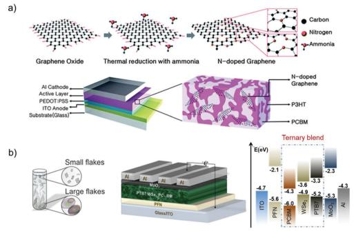
Fig. 8 (a) Schematic of the N-doping process of RGO and BHJ OSC using N-doped graphene/P3HT:PC<sub>61</sub>BM as the active layer. Adapted from ref. 572. (b) Schematic of the WSe2 flake production through LPE, and schematic of the device structure and energy levels. Adapted with permission from ref. 336, Copyright 2017, American Chemical Society.
