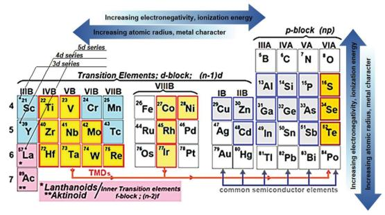
Fig. 2 Selected elements across the periodic table that—as a single element (e.g., Si, Ge), compounds (e.g., GaAs, CdAs), or alloys (e.g., Si<sub>x</sub>Ge<sub>1-x</sub>, Al<sub>x</sub>Ga<sub>1-x</sub>)—display semiconductor nature (into the blue frame) and the transition metals and three chalcogen (X) elements (enclosed by a red frame) that predominantly crystallize in layered TMDs. Partial highlights for Co, Rd, Ir, and Ni indicate that only some of their TMDs form layered structures.
