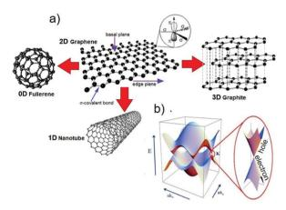
Fig. 3 (a) Schematic of the honeycomb graphene network as formed by C atoms and bonded basal  $\sigma$  bonds perpendicular to  $\pi$  orbitals. The other graphene-derived allotropes of C are also shown. Adapted from ref. 139 and 140. (b) Band structure in the honeycomb lattice. In the enlarged picture, the energy bands close to one of the Dirac points are also sketched. Adapted from ref. 141.
