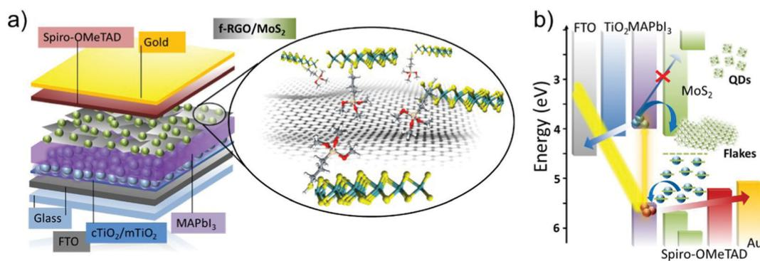
Fig. 22 (a) Schematic of mesoscopic  $\text{MAPbI}_3$ -based PSC using  $\text{MoS}_2$  QDs:f-RGO hybrids as both HTL and active buffer layer. (b) Schematic of the energy band edge positions of the materials used in different components of the assembled mesoscopic  $\text{MAPbI}_3$ -based PSCs. Reprinted with permission from ref. 1191, Copyright 2018, American Chemical Society.
