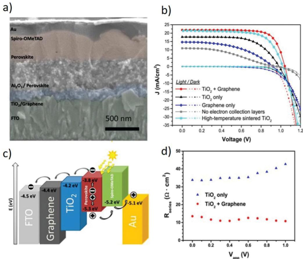
Fig. 19 (a) Cross-sectional SEM image of a PSC based on a graphene–TiO<sub>2</sub> composite as the ETL. (b)  $J$ – $V$  curves measured for PSCs with different ETLs under solar irradiation and in the dark (c). Energy levels of a PSC based on a graphene–TiO<sub>2</sub> composite as the ETL. (d) Series resistances of PSCs using pristine TiO<sub>2</sub> and graphene–TiO<sub>2</sub> composite as the ETLs. Reprinted with permission from ref. 1100, Copyright 2013, American Chemical Society.
