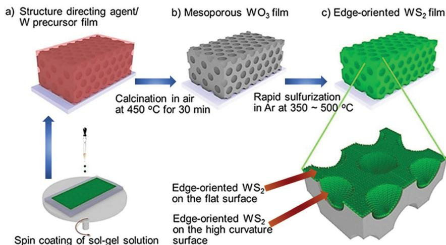
Fig. 15 Schematic of the preparation of solution-processed mesoporous WO<sub>3</sub> thin film and its conversion to edge-oriented WS<sub>2</sub> thin film. Adapted from ref. 839.
