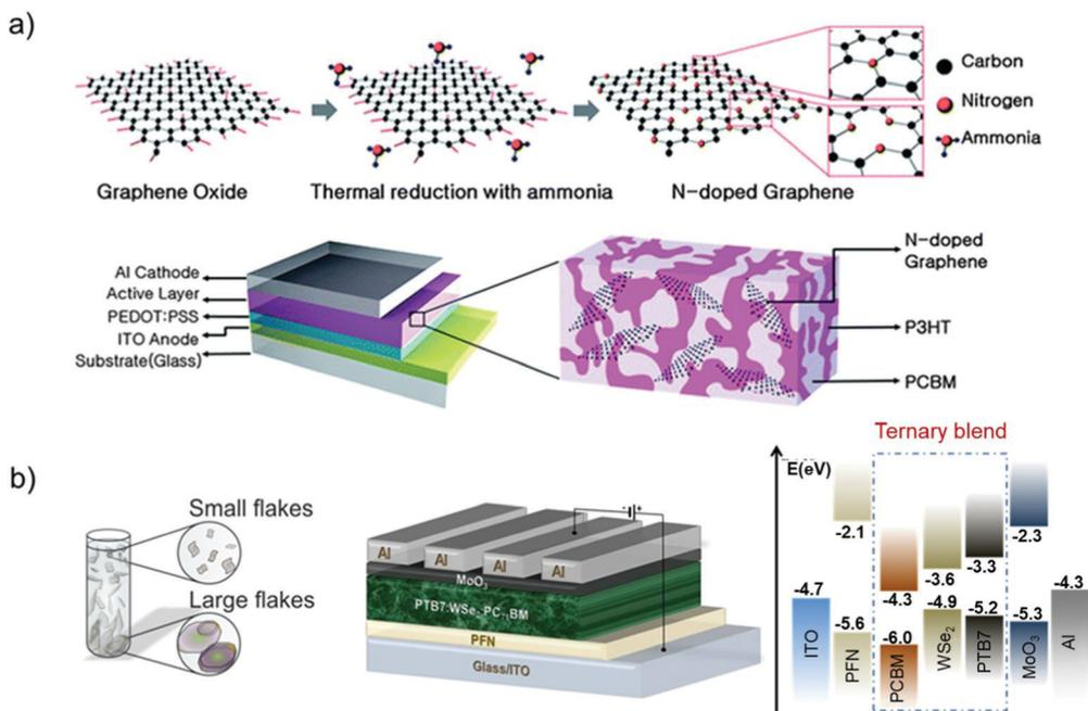
Fig. 8 (a) Schematic of the N-doping process of RGO and BHJ OSC using N-doped graphene/P3HT:PC<sub>61</sub>BM as the active layer. Adapted from ref. 572. (b) Schematic of the WSe<sub>2</sub> flake production through LPE, and schematic of the device structure and energy levels. Adapted with permission from ref. 336. Copyright 2017, American Chemical Society.
