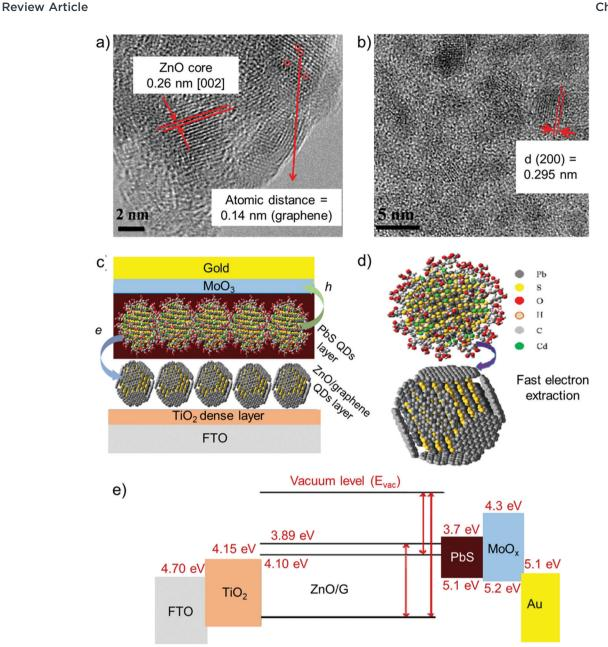
Fig. 27 High-resolution TEM images of (a) graphene QDs and (b) ZnO/graphene QDs. (c) PbS QD and ZnO/graphene QD-based depleted heterojunction QDSCs. (d) Schematic of the electron extraction process from PbS QD to ZnO/graphene QD. (e) Energy-level diagram of PbS QDand ZnO/graphene QD-based depleted heterojunction QDSCs (G = graphene). Adapted from ref. 1370.
