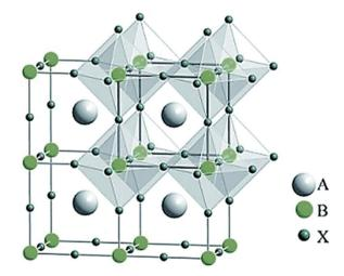
Fig. 17 The basic perovskite structure (ABX<sub>3</sub>). Adapted from ref. 899.
