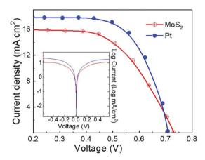
Fig. 16 J-V curves of DSSCs with MoS<sub>2</sub>/FTO and Pt/FTO CEs. Inset shows the Tafel polarization curves of symmetrical cells with MoS<sub>2</sub>/FTO and Pt/FTO CEs. Adapted from ref. 840.
