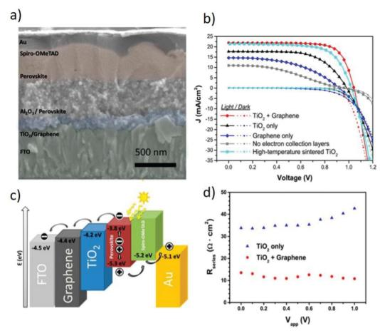
Fig. 19 (a) Cross-sectional SEM image of a PSC based on a graphene $-\text{TiO}_2$  composite as the ETL. (b) J-V curves measured for PSCs with different ETLs under solar irradiation and in the dark (c). Energy levels of a PSC based on a graphene-TiO2 composite as the ETL. (d) Series resistances of PSCs using pristine TiO2 and graphene-TiO2 composite as the ETLs. Reprinted with permission from ref. 1100, Copyright 2013, American Chemical Society.
