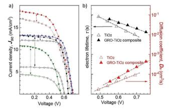
Fig. 14 (a) Typical J-V curves of DSSCs based on different GRM-based photoactive layers (line and full symbols) compared to those of the corresponding traditional TiO2-based photoelectrode. (b) Electron diffusion coefficient  $(D_n)$  and lifetime  $(\tau)$  dependence on the applied voltage for DSSCs based on TiO<sub>2</sub> photoactive layers with and without GRMs. Adapted from ref. 741,742,758,759.
