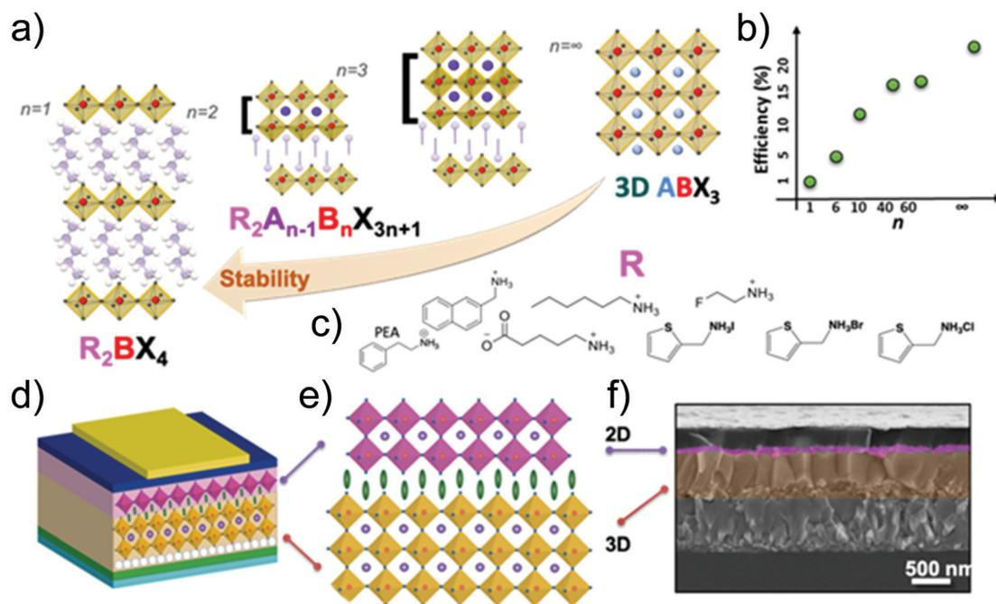
Fig. 25 (a) Structure of perovskite from 2D to 3D forms. (b)  $\eta$  versus  $n$ . (c) Typical cations used as R for the 2D perovskite formulation. (d) Structure of an  $n-i-p$  PSC based on FTO; cTiO<sub>2</sub>, mTiO<sub>2</sub>, 3D/2D perovskite, organic HTM, and Au CE. (e) Schematic of the 3D/2D active perovskite layer. (f) Cross-sectional SEM image of the 2D/3D device.
