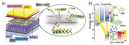
Fig. 22 (a) Schematic of mesoscopic MAPbl<sub>3</sub>-based PSC using MoS<sub>2</sub> QDs:f-RGO hybrids as both HTL and active buffer layer. (b) Schematic of the energy band edge positions of the materials used in different components of the assembled mesoscopic MAPbl3-based PSCs. Reprinted with permission from ref. 1191, Copyright 2018, American Chemical Society
