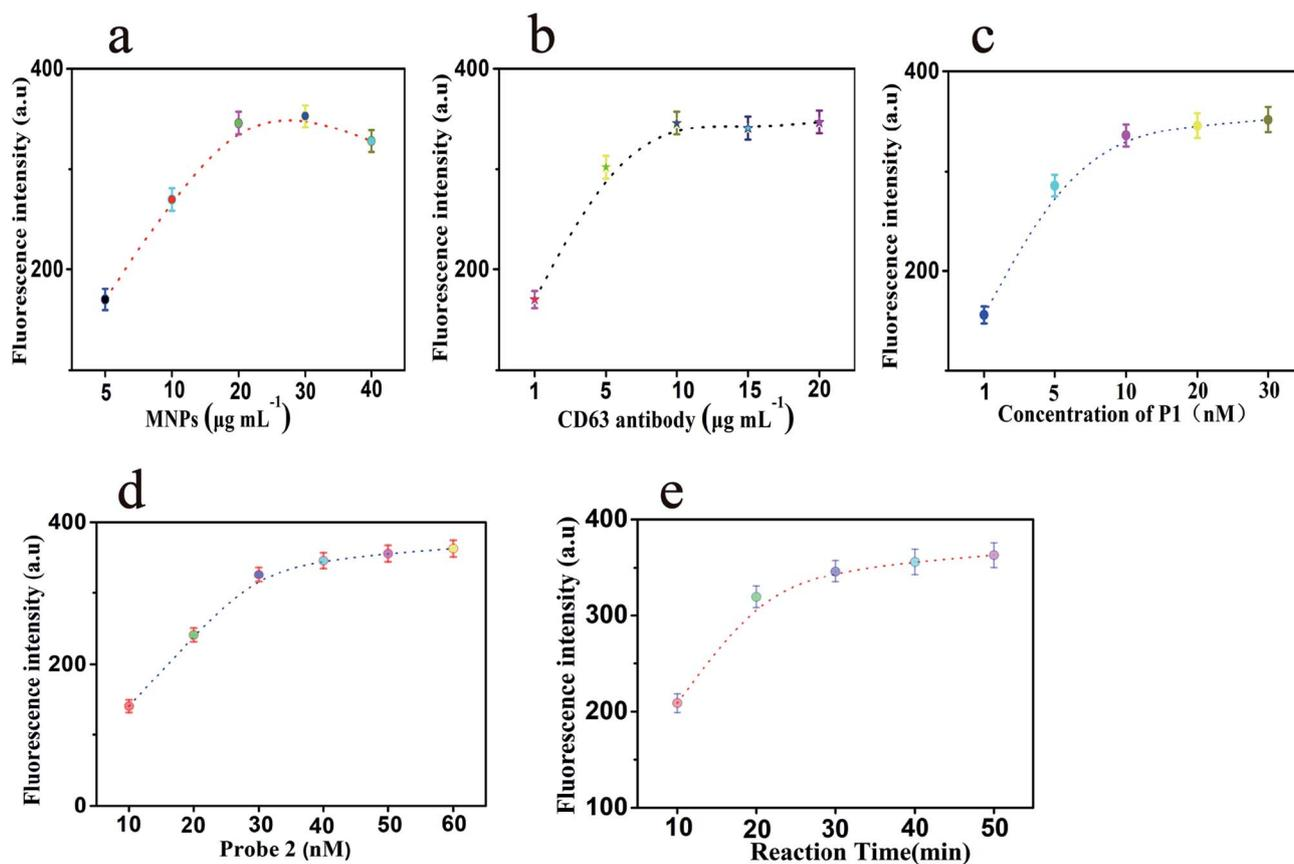
Fig. 3 Effects of the reaction parameters on the fluorescence signals of the proposed method: (a) the concentration of MNPs ( $\mu\text{g mL}^{-1}$ ), (b) the concentration of CD63 antibody ( $\mu\text{g mL}^{-1}$ ), (c) the concentration of P1 (nM), (d) the concentration of probe 2 (nM) and (e) reaction time (min). The lines represent the fluorescence intensity at different conditions. Error bars: SD,  $n = 3$ .
