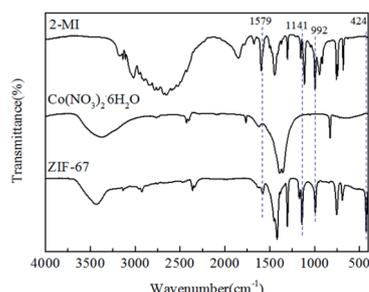
Fig. 3 FTIR spectra of 2MI,  $\text{Co}(\text{NO}_3)_2 \cdot 6\text{H}_2\text{O}$  and ZIF-67.
