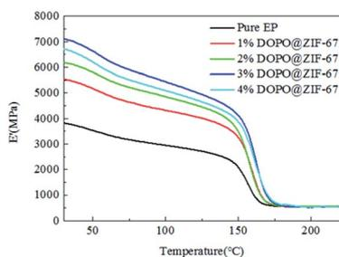
Fig. 15 The storage modulus of flame-retardant EP composites.
