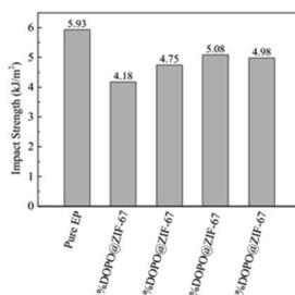
Fig. 18 The impact strength of EP composites.
