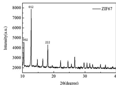
Fig. 4 XRD spectra of ZIF-67.
