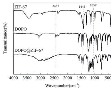
Fig. 6 FTIR spectra of ZIF-67, DOPO and DOPO@ZIF-67.
