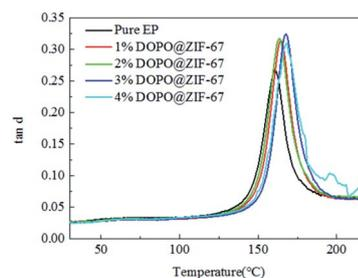
Fig. 17 The tan delta of flame-retardant EP composites.
