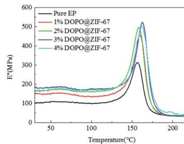
Fig. 16 The loss modulus of flame-retardant EP composites.
