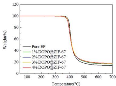
Fig. 9 TGA curves of pure EP and DOPO@ZIF-67/EP.
