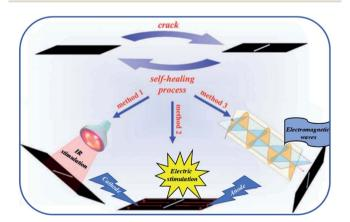
Fig. 13 Graphene–polyurethane composite healed under infrared, electric and electromagnetic stimulus.<sup>115</sup>
