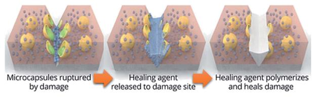
Fig. 2 Concept of self-healing based on microencapsulated healing agent (in yellow) embedded in a matrix (in red) containing a catalyst (in blue) capable of polymerizing the healing agent (in green). 10,111
