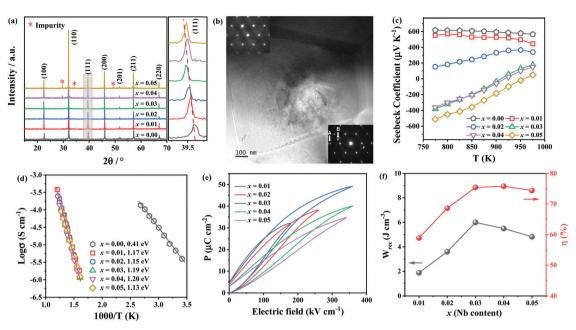
Fig. 3 (a) XRD patterns, (b) TEM image obtained from x = 0.03, (c) Seebeck coefficients, (d) Arrhenius plots of conductivity obtained from M'' peaks, (e) unipolar P-E loops under  $E_{max}$ , and (f) the energy storage properties,  $W_{rec}$  and  $\eta$  of BF-ST-BMN-xNb.
