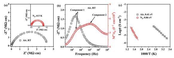
Fig. 2 (a) Z\* plots of the air sintered 0.54BF-0.4ST-0.06BMN ceramic at RT and the N<sub>2</sub> sintered ceramic at 613 K as inserted, respectively; (b) Z" and M" spectroscopic plots at RT of the ceramic sintered in air; (c) the Arrhenius plots of conductivity extracted from M'' plots for ceramics sintered in air and  $N_2$ .
