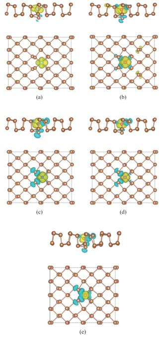
Fig. 5 Top view of spin density of doped antimonene: (a) Ti–Sb, (b) V–Sb, (c) Cr–Sb, (d) Mn–Sb, and (e) Fe–Sb. The isosurface value is set to be  $0.0015e~{\rm \AA}^{-1}$ .
