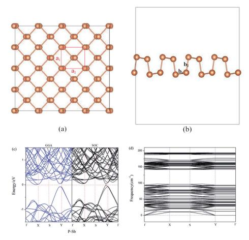
Fig. 1 The top (a) and side (b) view of the optimized structure of pristine antimonene. (c) Band structure and (d) phonon dispersion curves structure of pristine antimonene.
