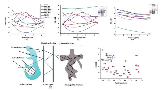
Fig. 12 EMI shielding of composite (a) SE, (b) SE<sub>A</sub>, (c) SE<sub>R</sub>, (d) EMI shielding mechanism and (e) EMI shielding comparison.
