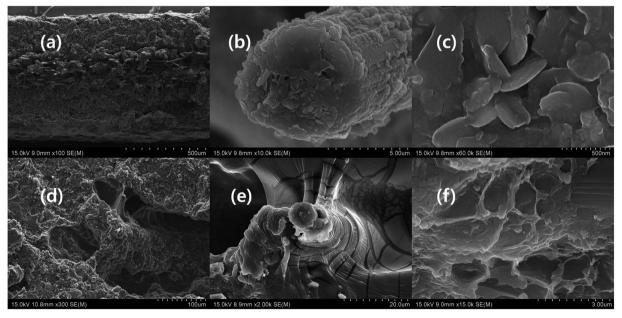
Fig. 6 Cross-section of composite (a) MXAPPA, (b) MXene on carbon fiber (×10 000), (c) MXene on carbon fiber (×60 000), (d) MXPATPPy, (e) uMXPAT, and (f) rMXPAT.
