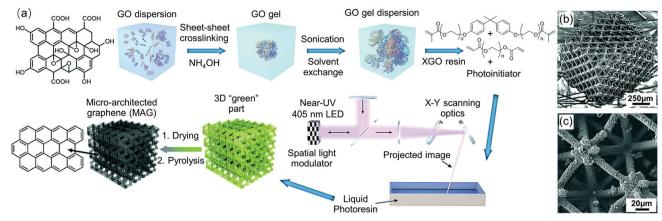
Fig. 12 Fabrication of PmSLA printed graphene aerogels using photo-activated GO resin. (a) Schematic illustration of a synthesis process of microarchitectured graphene (MAG). (b) and (c) SEM images of crosslinked GO particle (XGO)-derived MAG. Adapted from ref. 244 with permission from the Royal Society of Chemistry
