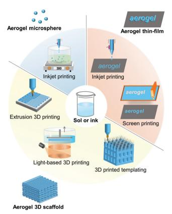
Fig. 4 Commonly employed printing technologies for aerogels: inkjet printing for microspheres, inkjet and screen printing for patterned thin-films and extrusion, light-based printing, or 3D printed templates for 3D aerogel structures
